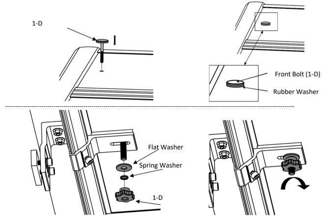
**XATTENTION:** Make sure the Flat Washer and Spring Washer are all placed on bolt before screw the plastic nut on.
