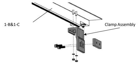
Step-2 Attach and Install the other set of Clamp Assembly (1-G) to the Side Rail (1-B&1-C), then tighten the nuts.
