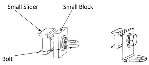
Insert the small slider into the Track Channel. Tighten the bolt. (Note: Make sure the small slider isinstalled nearby the Strap Safety Buckle position) There is a hole on the bottom of the bolt. Snap the safety buckle into the hole of the bolt.
