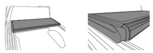
8. Adjust the front support plate(1-F) to correct position, insert the front bolt with rubber washer into the holes on the cover front panel and front support plate. Then tighten the hand nut under the front support plate.
