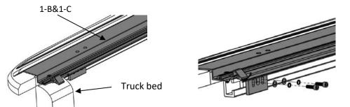
7. Place the bed cover on the front end of truck bed. Ensure the cover is even on all sides and sit firmly on side rails.
