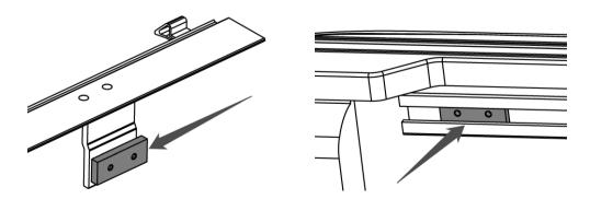
6. Place the side rail on the bed rail, and push it to the front wall of truck bed. Then bolt the side rail with the aluminum block (already in the Factory Track in Step 5) together. Tighten the clamps each side.
