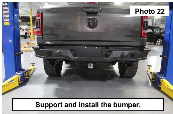
19. Secure the bumper using (2) of the supplied flag nuts and (2) 12mm hex head bolts and (2) 12mm flat washers Per side to secure the rear bumper. Tighten using a 19mm socket. **See Photo 23.**
