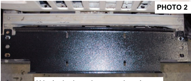
YJ winch plate placement location.
