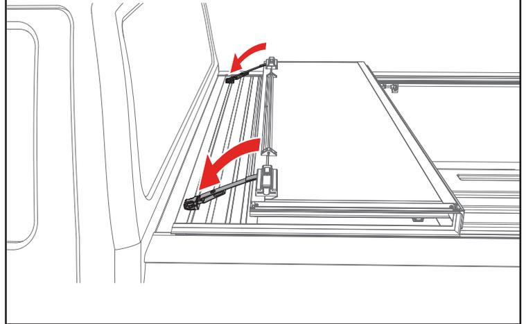
**FLIPPED UP POSITION:** Fold the cover (A) open and lift it until it's vertical towards your truck cab. Then release the prop rod that is attached to the side rail and clip it onto the ball stud on the underside of the cover.
