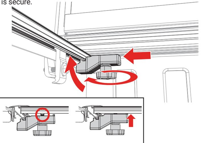
**15** Unfold the cover (A) towards the tailgate. Then confirm each panel is centered side to side and front to back on the truck bed. If adjustments are needed, loosen the cover retainer clamps (G) and shift the cover (A) until positioned correctly. Retighten the cover retainer clamps once the desired fitment is reached. *If adjustments to the slam latch are needed, see the directions on the next page.*
