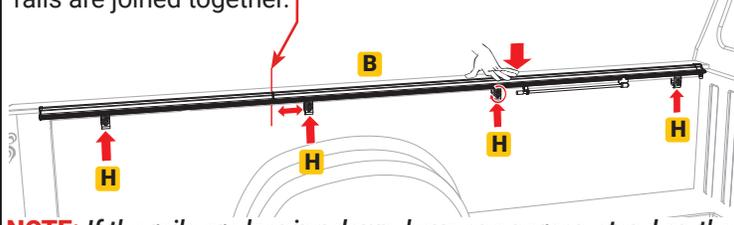
**NOTE:** If the rails are leaning down, have one person stand on the outside of the bed and slightly roll the rails upward while another person slowly snugs the clamps up. If the clamps are tightened too quickly or overtightened, it will cause the rails to lean down.
