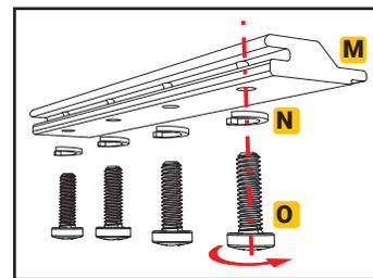
Then slide the assembled rail coupler (M) into the bottom end of the driver side rail (B) section as shown.
