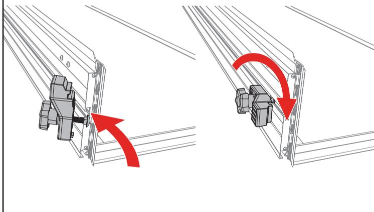
**12** Position the buckle ends (I) with the open side facing the bed cover panel. Use a screwdriver to install the two buckles into the pre-drilled holes on the front header panel with the provided screws (J). **DO NOT use a screw gun, securely tighten by hand only.**
