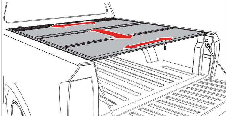
**16** The rear edge of the cover (A) and tailgate seal should rest on top of the tailgate. **You are ready to drive with your cover in the closed position.**
