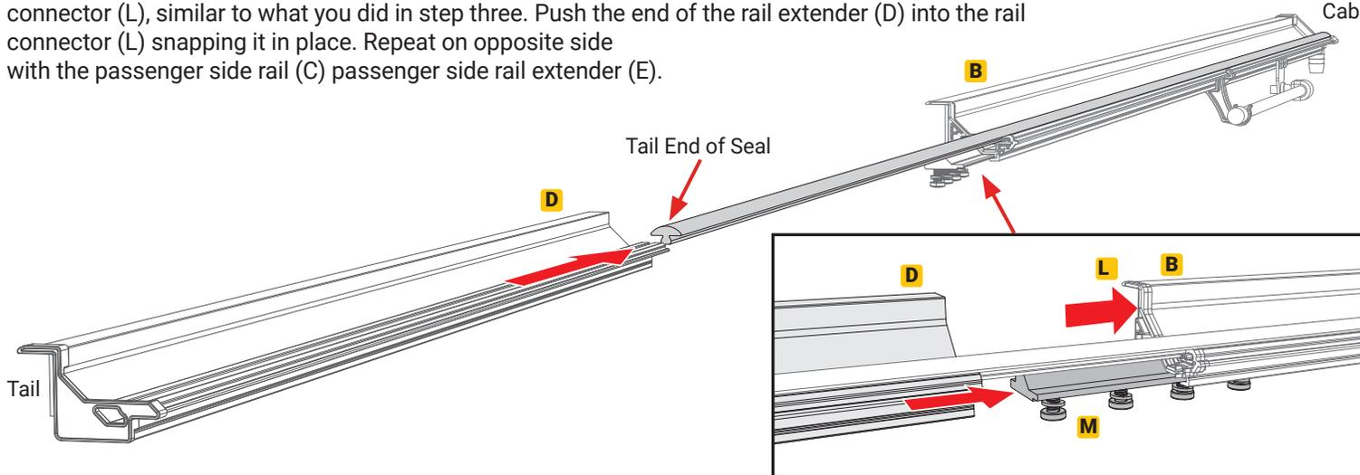
**5** After both rail sections are slid together, tighten both screws (O) on the driver side rail (B) with a Phillips screwdriver. Repeat on passenger side.
