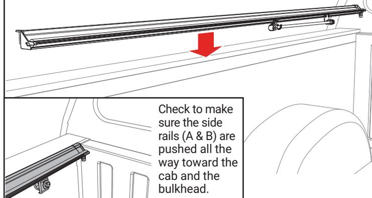
Check to make sure the side rails (A & B) are pushed all the way toward the cab and the bulkhead.
