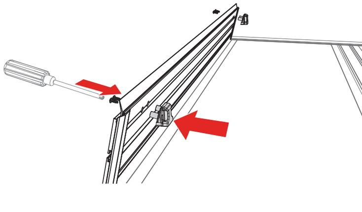
**13** Set the cover (A) in the folded position on the side rails (B & C) towards the cab of the truck. Confirm the cover is evenly spaced between the rails.
