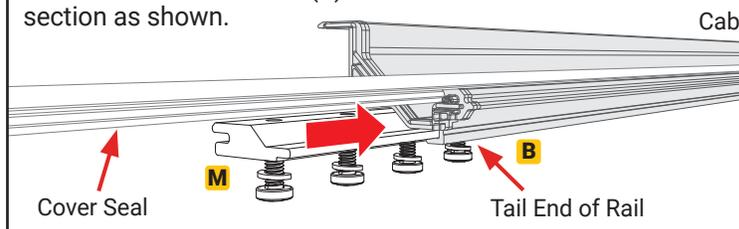
**4 Installing Rail and Rail Extender:** Slide driver side rail extender (D) on to the tail end of the seal pushing the rail toward the driver side rail (B). The bottom end of the driver side rail extender (D) slides into the rail coupler (M) and then into the rail connector (L), similar to what you did in step three. Push the end of the rail extender (D) into the rail connector (L) snapping it in place. Repeat on opposite side with the passenger side rail (C) passenger side rail extender (E).
