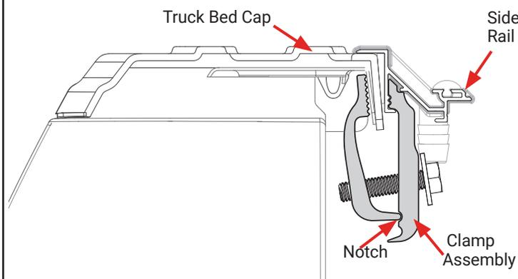
**11** Before placing the cover (A) onto the vehicle, slide two front cover retainer clamps (G) into the track on the underside of the cover (A) near the cab. Confirm the cover retainer clamps fit properly into the cover rail for optimum fit. Repeat on the opposite side of the cover.
