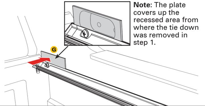
**Note:** The plate covers up the recessed area from where the tie down was removed in step 1.
