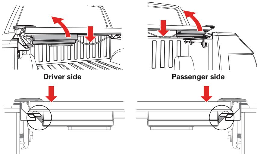
**15** Retighten the cover retainer clamps once the desired fitment is reached. **You are ready to drive with your cover in the closed position.**
