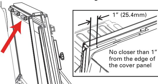
**12** Clean the tailgate extrusion of the hard fold cover (A). Then peel the backing from the tailgate seal (P) and adhere the seal from one tailgate extrusion edge to the other. Apply pressure evenly to the entire seal to ensure proper adhesion.
