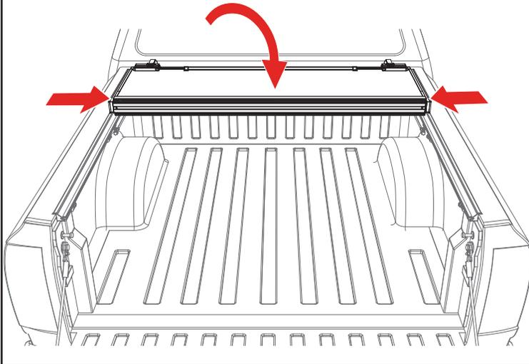
**10** Confirm the retainer clamps (E) are positioned around the side rails (B & C) correctly as shown below. Tighten the retainer clamps by turning them clockwise until the lock washer is secure.
