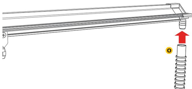
**6** Route the other end of the drain tube (O) through the tie-down hook and into the factory bed plug. Remove this plug first or drill a 7/8" hole through the plug. Alternately, the plug can be cut using a utility knife, making sure to cut a hole large enough to not crimp the drain tube. **NOTE:** If you have a drop-in bedliner, just route the drain tubes behind the liner. Repeat on the driver's side.
