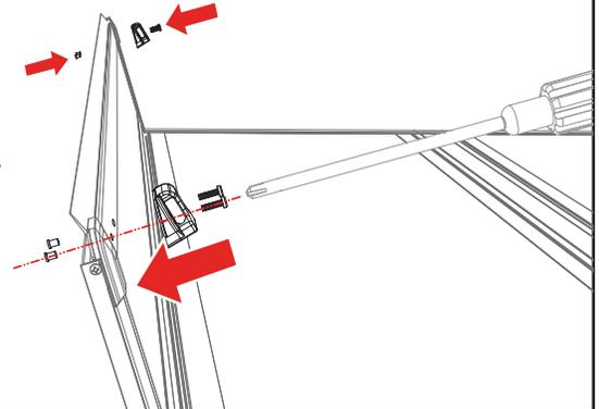
**9** Set the cover (A) in the folded position on the side rails (B & C) towards the cab of the truck. Confirm the cover is evenly spaced between the rails.
