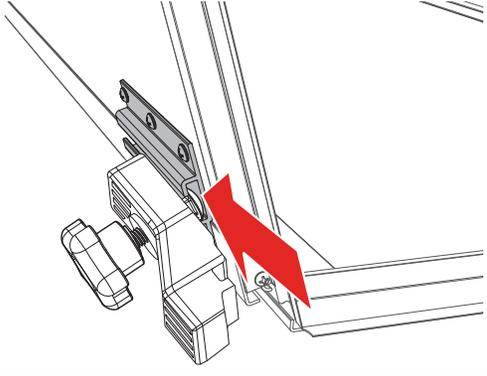
**8** First, prep the buckle ends (H) by peeling off the adhesive liner of the gasket (I). Then adhere the gasket (I) to the underside of each of the buckle ends.
