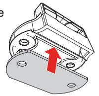
Position the buckle ends (H) with the open side facing the bed cover panel. Use a Phillips screwdriver to install the two buckles into the pre-drilled holes on the front header panel with the provided screws (J) and the nutsert (K) inserted from the backside of the panel. **DO NOT use a screw gun, securely tighten by hand only.**
