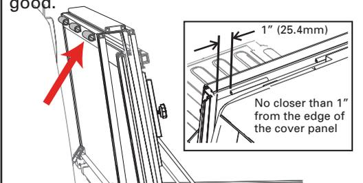
**23** Unfold the cover (A) towards the tailgate. Then confirm each panel is centered side to side and front to back on the truck bed. If adjustments are needed, loosen the cover retainer clamps (G) and shift the cover until positioned correctly. The rear edge of the cover and tailgate seal should rest on top of the tailgate. For proper sealing, the tail panel will overlap by .5".
