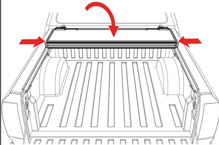
**21** Confirm the retainer clamps (G) are positioned around the side rails (B & C) correctly as shown below. Tighten the retainer clamps by turning them clockwise until the lock washer is secure.
