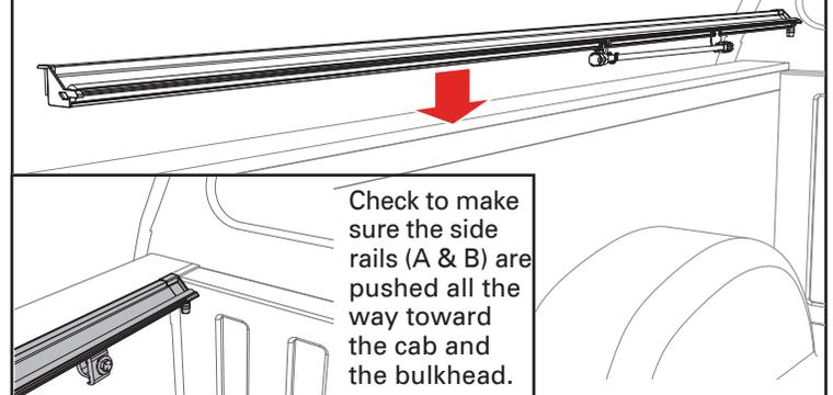
Check to make sure the side rails (A & B) are pushed all the way toward the cab and the bulkhead.
