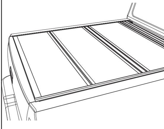
**OPENING COVER:** Lower the tailgate and pull the cable on either side. While pulling on the cable lift the panel up and towards the cab.
