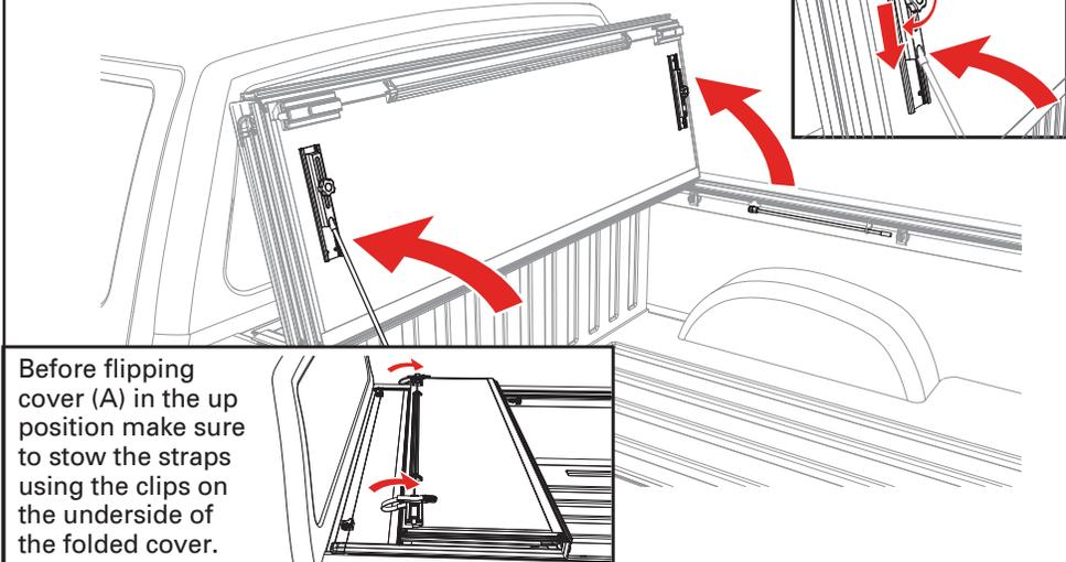
Before flipping cover (A) in the up position make sure to stow the straps using the clips on the underside of the folded cover.
