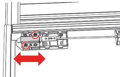
With the latch cover removed, loosen the screws and move the latch bracket to adjust. Retighten the screws. Slide the latch housing back on.
