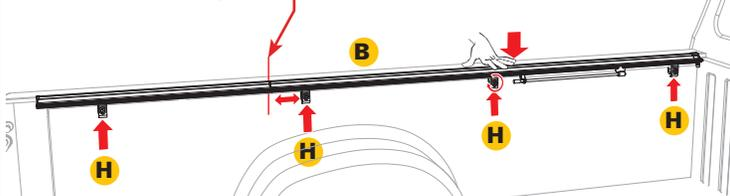
**NOTE:** If the rails are leaning down, have one person stand on the outside of the bed and slightly roll the rails upward while another person slowly snugs the clamps up. If the clamps are tightened too quickly or overtightened, it will cause the rails to lean down.
