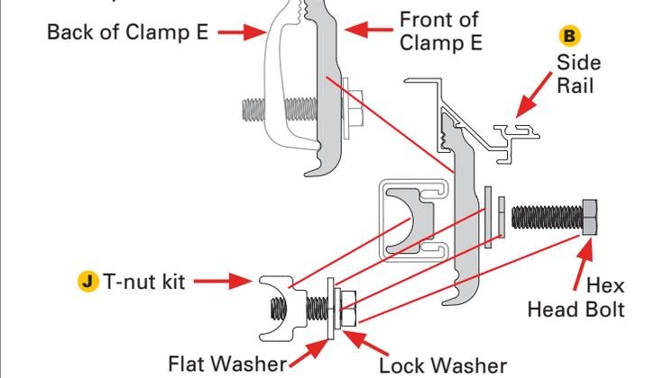
**13** Installing T-nut Kits in Cargo Management System: Remove the factory end cap from tailgate end of the accessory rail. Insert three T-nut kits (J) into the end of the accessory rail and put the end cap back in. Repeat on passenger side.
