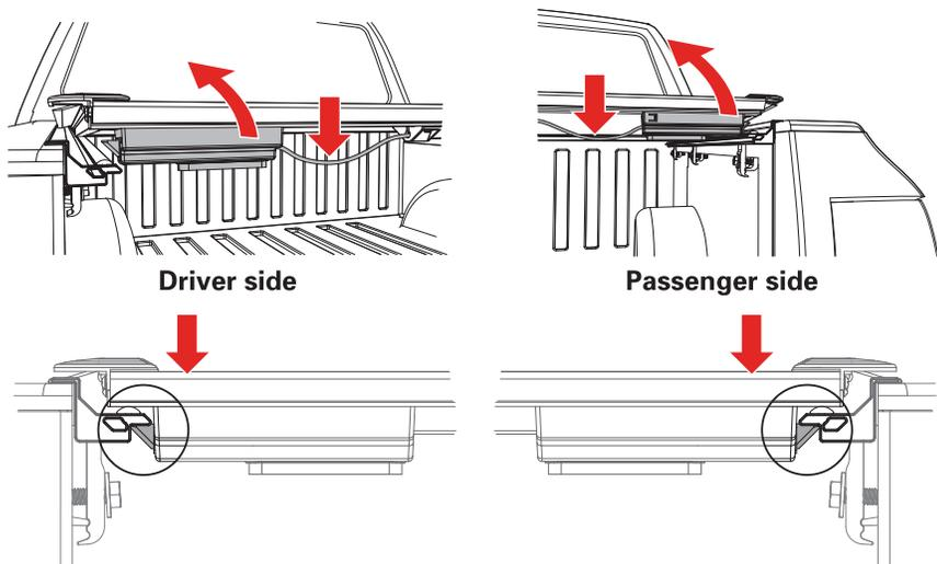
**25** Retighten the cover retainer clamps once the desired fitment is reached. **You are ready to drive with your cover in the closed position.**
