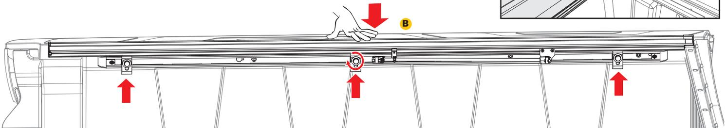
**NOTE:** If the rails are leaning down, have one person stand on the outside of the bed and slightly roll the rails upward while another person slowly snugs the clamps up. If the clamps are tightened too quickly or overtightened, it will cause the rails to lean down.
