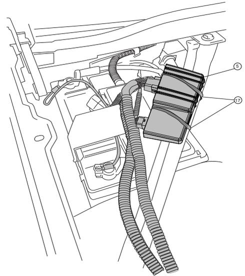
Remove power fuse. Attach power lead (RED wire) to positive pole on the battery. Attach ground lead to negative battery pole.
