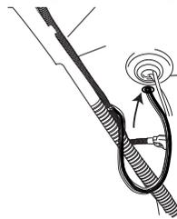
NOTE: Seal holes with silicone glue and cover with tape so carpet does not stick to glue.
