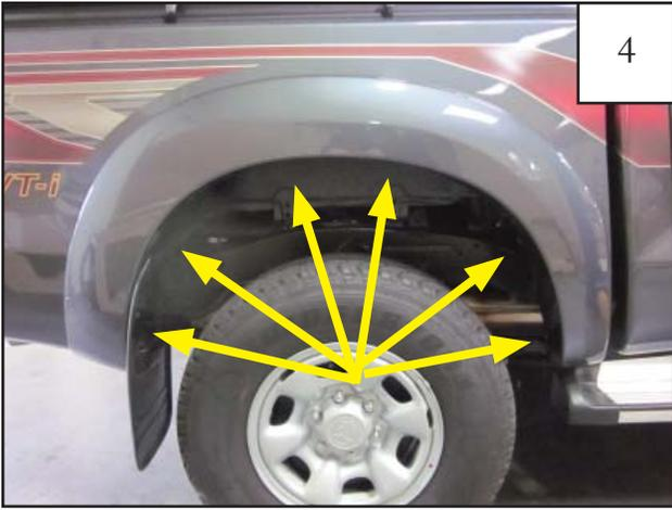
Remove six factory screws from the fender lip. Save screws for reinstallation. Remove flare by pulling part away from side of vehicle.
