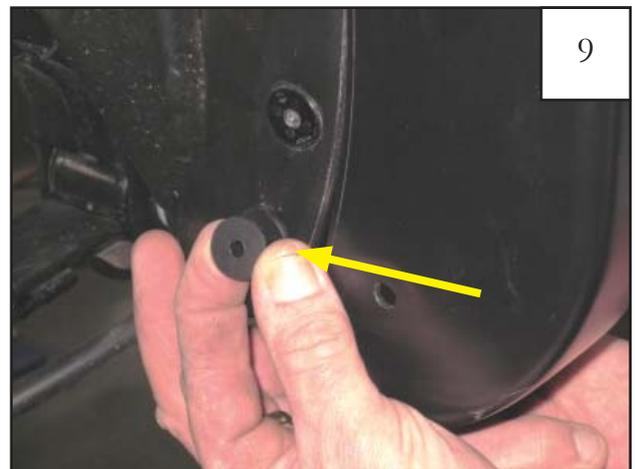
Install supplied grommet (GR1-0001) into factory hole.
