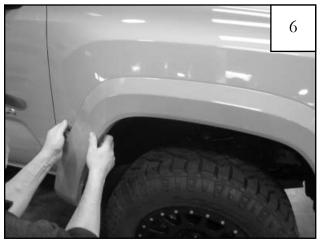
Remove flare by pulling part away from side of vehicle
