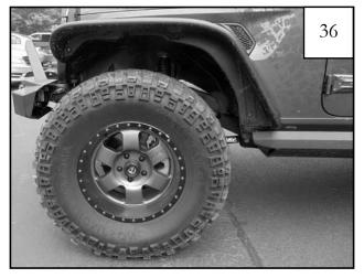
Completed front driver's side flare installation.
