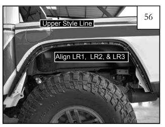
Ensure that inner pieces LR1, LR2, & LR3 are aligned together properly, and tighten all allen head bolts. *Inner piece should rest along upper style line of sheet metal radius and not below it.*
