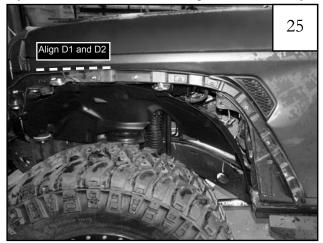
Ensure that inner pieces D1 and D2 are aligned together properly, and tighten all allen head bolts.
