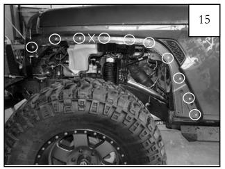
Ten rivnuts installed. NOTE: The "X" above indicates a hole that is not used.
