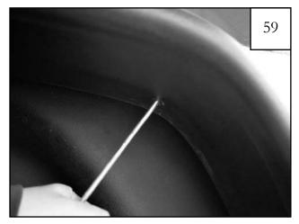
Use a scratch awl (or another pointed tool) to line up the U-clips with the outer flare holes (9 locations). If needed, use a flashlight to better locate the speed clips.
