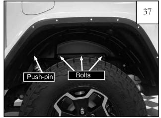
Using a pry tool, pliers, or flat head screwdriver, remove (3) 8mm bolts and (1) push-pin from inside of splash shield.
