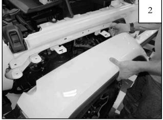
Starting at front of flare, pull *firmly* to release flare and splash shield from fender, working your way to the back. You will hear popping noises as clips release. It is okay. If clips break, they will be discarded. Clip off both socket connectors at the existing light.
