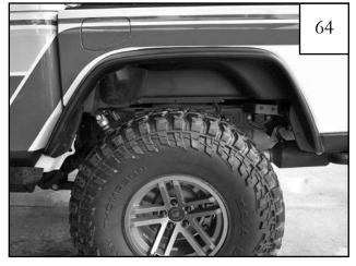
Completed rear driver's side flare installation.
