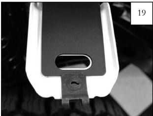
Install a U-clip on both flanges of the support bracket.
