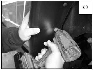
Hold flare in place on fender and **START** a SW1-0057 Phillips Truss Screw into each hole location and through the U-clip on inner structure (9 locations). **DO NOT TIGHTEN.**
