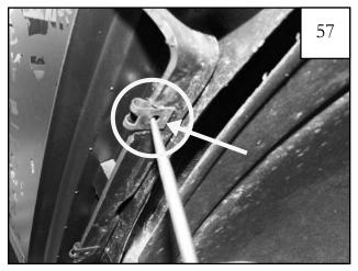
Before installing the outer flare, make sure that the CL1-0022 U-clips on the inner pieces are centered over the predrilled holes.
