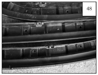
Locate the flat flare rear inner pieces. The driver side rear inner pieces are marked LR1, LR2 & LR3.
