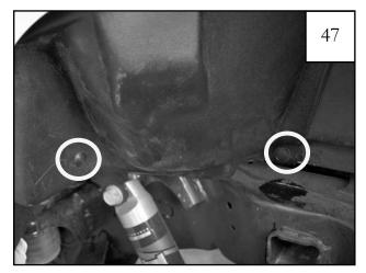
Position the Protective Case over the front wiring harness. Press the exposed tape liner against the side surface to tack it in place. Install the Protective Case in place using the fasteners.
