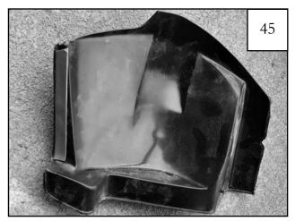
Remove the red tape liner from the Protective Case for the front wiring harness and fuel filler lines.
