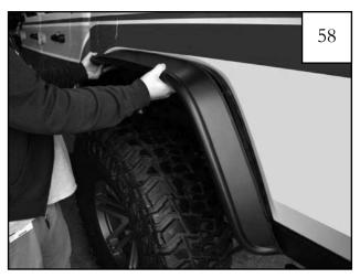
Place the outer flare over the inner pieces and push until snug against the vehicle surface.
