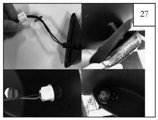
Front Turn Signal Install: remove plastic nut and lock washer from light. Slide stem through hole in front of fender flare. Add lock washer and nut back to the light behind the fender flare and tighten down. Side Marker Light: Push round button light through the hole under the lip of the fender flare.
