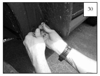
Use a scratch awl (or another pointed tool) to line up the speed clips with the outer flare holes (9 locations). If needed, use a flashlight to better locate the speed clips.
