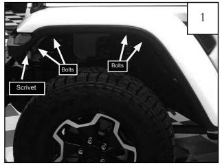
Remove and retain bolts and scrivet fastener from inside of factory fender.
