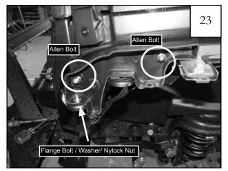
**Step 2** Slide a washer onto allen bolt. Insert a bolt/ washer assembly through inner piece and fender and secure to rivnut. *Start the bolts but do not tighten*. Next, install a 1/4-20 flange bolt and washer with nyloc nut as indicated above. Tighten this bolt fully.
