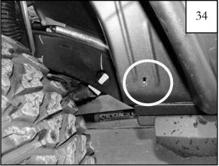
Install a RV1-P006 8-20mm nylon retainer in lower inside corner of fender flare.
