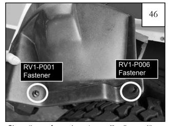
Clean the surface where tape will adhere with an alcohol pad. Press the exposed tape liner against the rear surface to tack it in place. Place (1) RV1-P001 fastener and (1) RV1-P006 fastener in place on the Protective case as shown.
