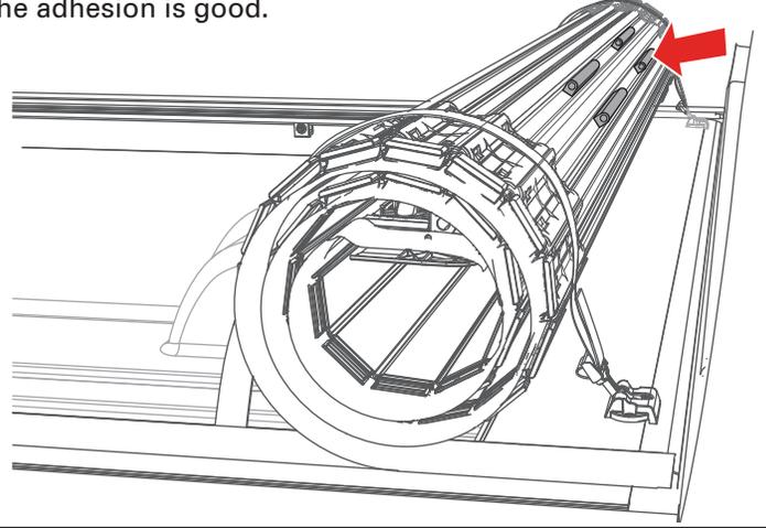
**Note:** If the side seals of the cover appear wrinkled, exposure to the sun will assist the seals to lay flat. Applying heat with a hair dryer or carefully with a heat gun will also smooth the seals.
