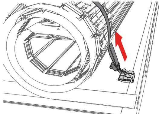
**Prior to vehicle operation, the truck bed cover MUST be properly secured.**
