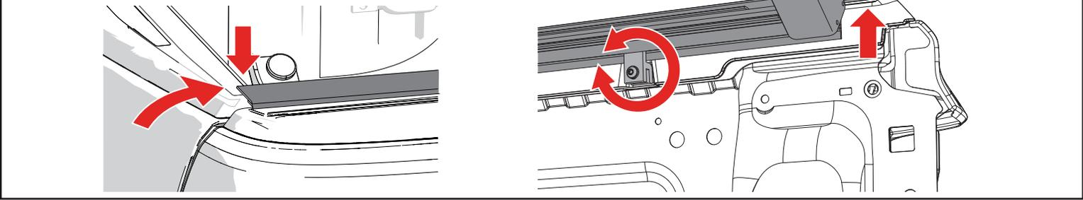
**7** With both rails (A & B) clamped in place, rest the rolled cover (C) onto the rails at the tailgate, roll the cover toward the cab, remove and discard all packaging materials.
