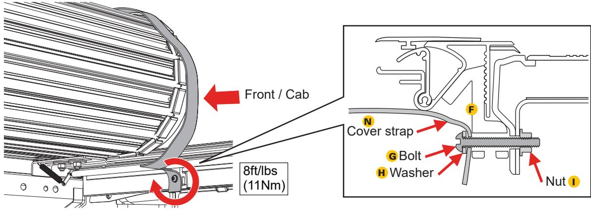
**4c - FOR 2025 RANGERS:** Install a rail clamp (P) at each point where the plastic clips were removed. Install the clamp up into the cover rail (A), making sure that it is inserted all the way up into the rail with the teeth of the clamp aligned with the slots in the rail. Insert a clamp bolt (G) through oversized washer (Q), through the clamp, and through the truck bed rail. Thread a clamp nut (I) onto the bolt.
