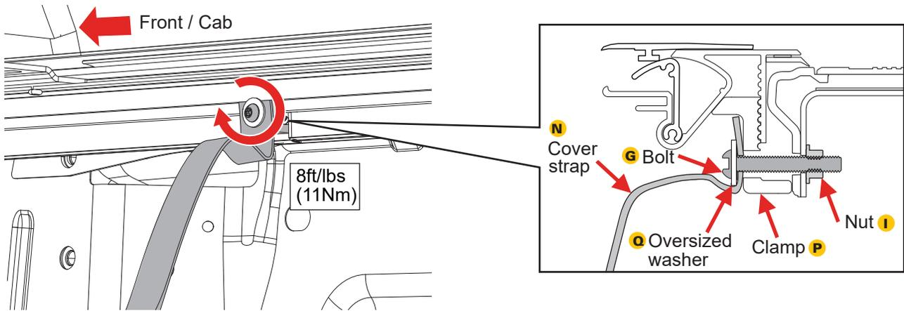
**5** Starting with the front clamp (F) for **2024 models** or front clamp (P) for **2025 models**, apply downward pressure to the cover rail (A & B) while tightening the bolt. Tighten to 8 ft/lbs (11 Nm) of torque. Repeat with the middle and then rear clamp, making sure that the rail is square and flat with the truck bed rail. Repeat steps 3-5 on the driver side.
