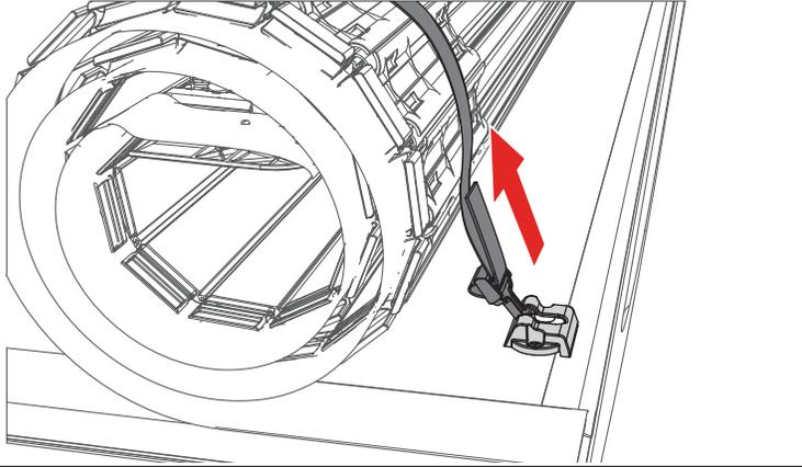
**18** With the cover (C) rolled open install the four D-shaped bumpers (O) to the cover slats.
