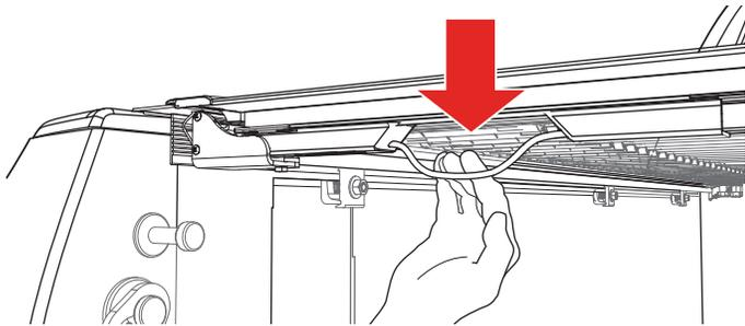
**ROLLED UP POSITION:** To drive with the cover (C) in the open position, use the cover straps (N). Roll the cover forward, twist and insert the clips into the cover clasps. Ensure that **BOTH** strap clamps are fully inserted into the clasps, pull on the end of the strap to tighten.
