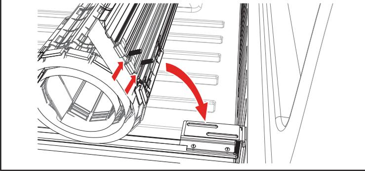
**10** Install the mounting hardware loosely underneath the slotted bracket on the passenger cover rail (A). Start with the rubber washer (L), then the large flat washer (K), then hand tighten the knobs (J). Repeat on the driver side. Leave the knobs loose for now.
