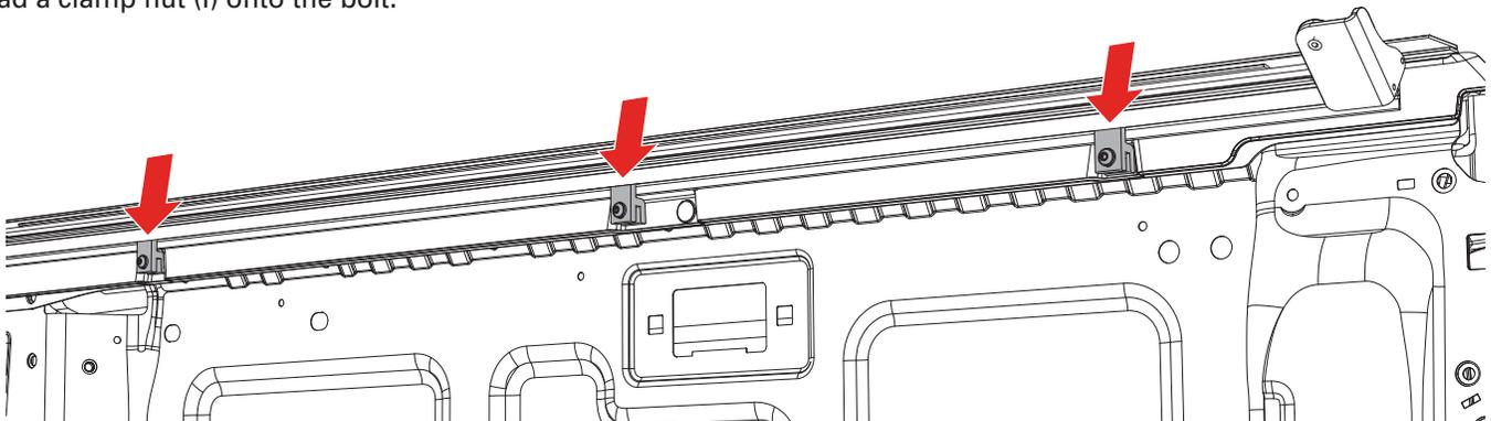
**4b - FOR 2024 RANGERS:** Mount the cover strap (N) to the forward most clamp (F) as shown. Use the provided washer (H) to retain the strap. Tighten to 8 ft/lbs (11Nm) of torque. Mount a strap to both sides.
