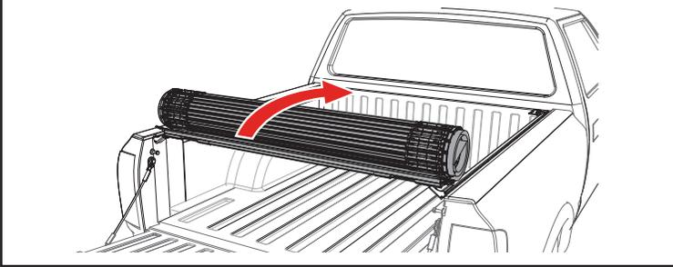
**8** Align the front vinyl edge of the cover (C) with the front edge of the cover rails (A & B) (not the rubber seal).
