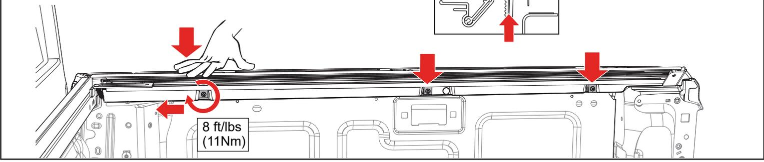
**6** With both cover rails (A & B) in place, check that the tailgate clears the overhanging edge of the cover rails on both sides. The edge of the cover rail may contact the tailgate cap. If this happens, loosen the rear clamp (F) for **2024 models** or the rear clamp (P) for **2025 models** and adjust the height of the rail. Re-tighten the clamps to the specifications in step 5.
