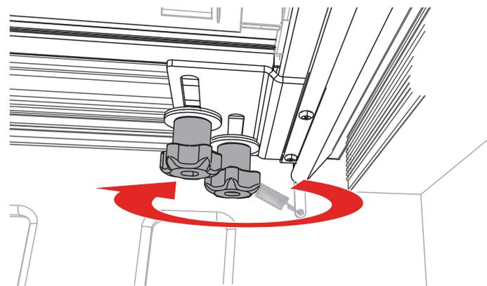
**17** The other end of the cover strap (N) inserts into the cover clasp and turns to lock.
