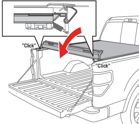
**COVER CLOSED:** The cover (C) must be **FULLY LATCHED ON BOTH SIDES** of the cover rails (A & B).
