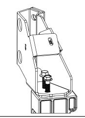
Remove support bar with a 21mm deep socket and a 13mm socket or wrench.
