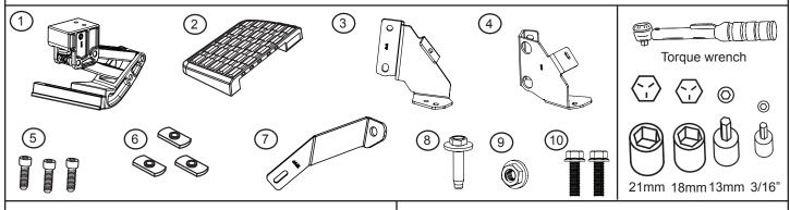
Assemble brackets as shown. 33 ft-lbs / 44 Nm
