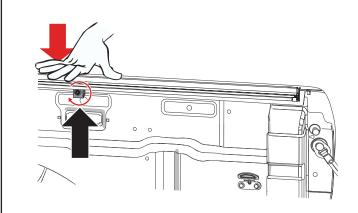
FOR TRUCKS WITH CARGO RAILS: Insert the second clamp (D) above the cargo rail near the tailgate. Slide the second clamp to approximately the center of the rail. Hand tighten the bolt enough to hold the clamp in place.
