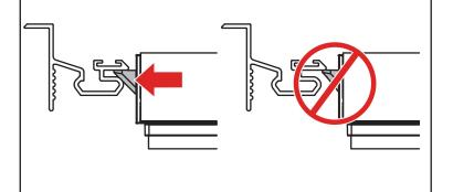
Once the cover (A) is properly aligned, carefully open the cover, ensuring that it remains in position. Tighten the four lock nuts (H). Do not over-tighten the fasteners. Do not use power tools. Check that the cover operates correctly and the latches engage. If not, loosen the fasteners and realign, starting from step 11. Also the tailgate latch itself can be adjusted in the next step.
