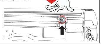
Tighten the clamps (D & E) starting with the middle, then the front and rear. Always apply downward pressure to the rail when tightening to ensure that the rail sits flush and seals properly. Repeat steps 2 - 6 for the driver side rail (B).
