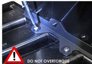
8. TIGHTEN WASHER/ SCREW MUDFLAP/BACKET ASSEMBLY BY HAND ONLY UNTIL WASHER IS SEATED
