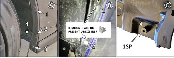
**FIGURE D** Position logo-side of flap facing rear of vehicle against liner mounts. Fasten 1SS and SMWASH to mounts 1 & 2, factory screw and SMWASH on point 3. For mount 4, install 2SS, SMWASH and SPACER **behind** mud flap.
