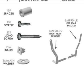
**Recommended Tools** Low-profile offset or ratcheting screwdriver, flathead screwdriver, needle nose pliers (optional). **Important Tips** Installation should be done on even surface. Do not use drill to tighten hardware. Hand tools only. Avoid overtightening.
