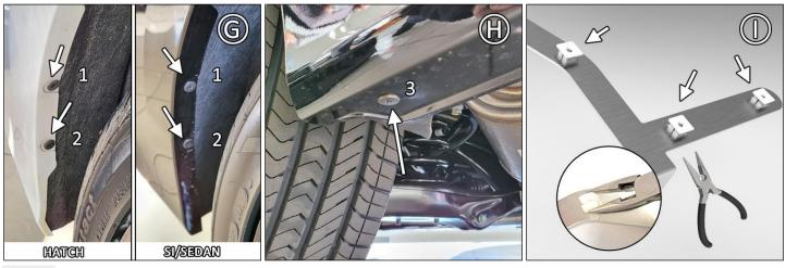
**FIGURE J** Position BMF90-RR/LR bracket behind bumper, over liner. Align upper mounts 1 and 2 on bracket to bumper mounting holes. Install original screw to mount 6.
