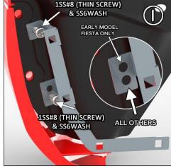
**FIGURE J** Refer to diagram J when positioning 4 x INS7 into rear bracket square mounts - Push INS7 in until **fully** seated.
