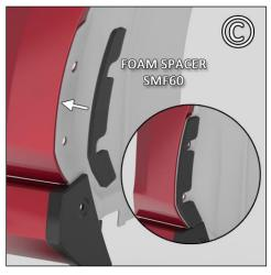
**FIGURE D** Place mud flap logo-side to the rear of the vehicle against mounting points on BRACKET#4 & liner. Pair WASH & 1SS to fasten mounts 1 & 2. Use a WASH & **MEDIUM SCREW** 1.5SS for point 3. Do not fully tighten.
