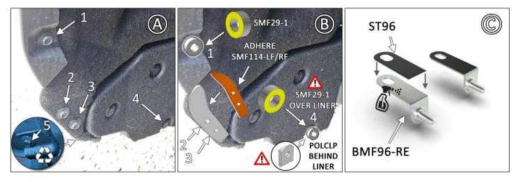
**IMAGE D** Place BMF96-RE over mount 5, then reinstall original fastener 5.
