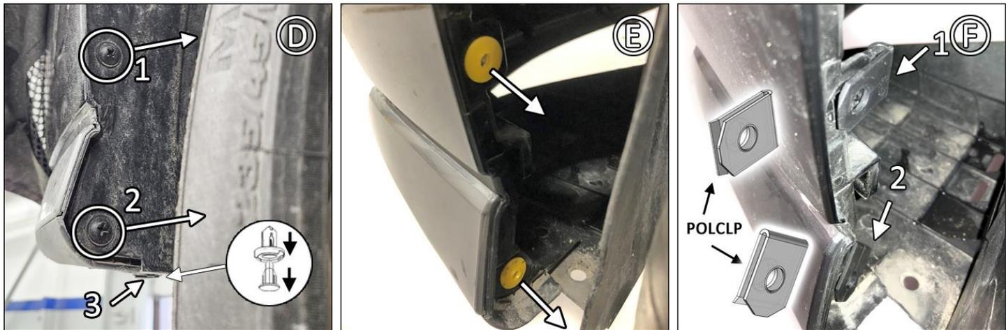
**FIGURE G** Reinstall factory fastener 3. Wipe area clean before adhering SMF103-LR/RR against mounting points.
