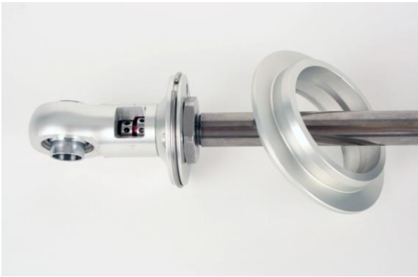
Figure 6 – Removing the Upper Spring Seat
