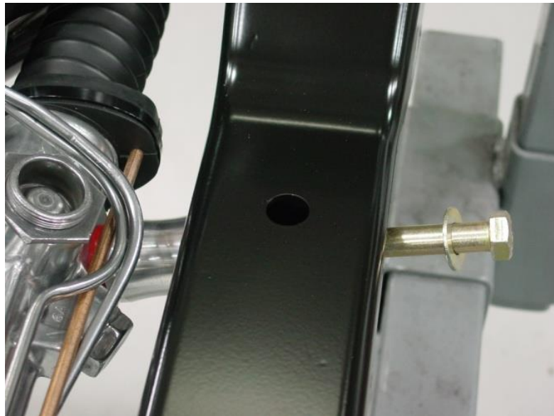
Figure 15 - Attaching the Rack to the Cross Member
