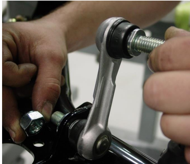
Figure 22 – Attach the End Link to the Lower Control Arm
