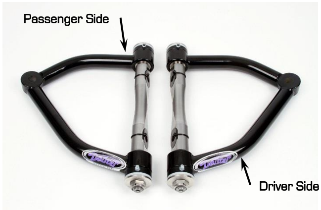
Figure 4a - Driver & Passenger Upper Control Arms
