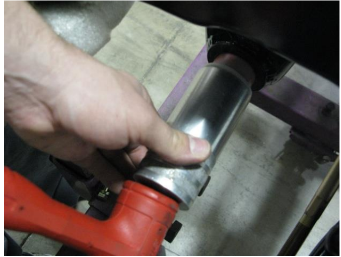
Figure 18 – Fully Installing the Bushings
