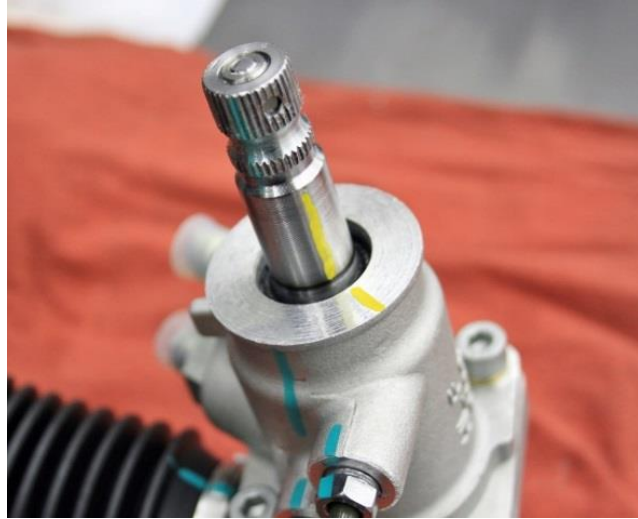
Figure 13 – Center the Rack & Pinion
