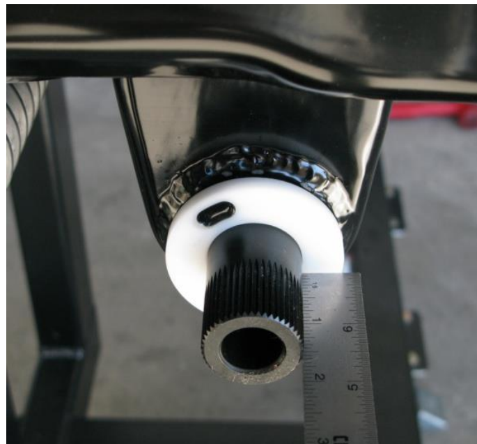
Figure 19 – Measuring the Sway Bar
