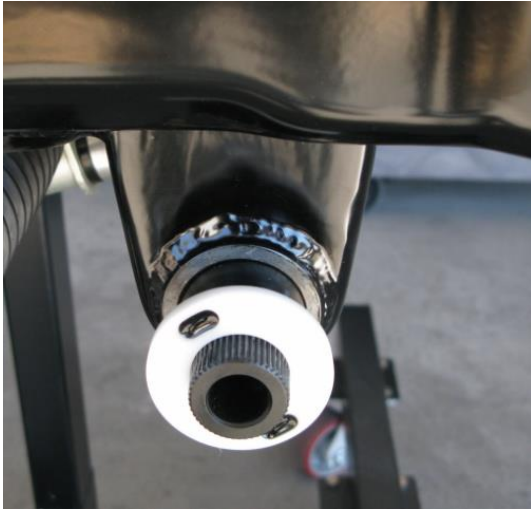
Figure 17 – Installing Bushing & Sway Bar
