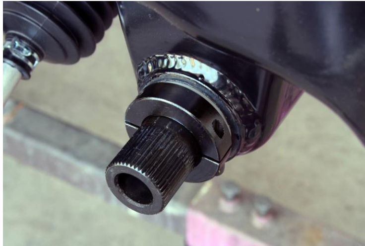
Figure 20 - Indexing the Clamp
