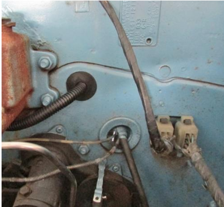
Figure 14 – Install Wiper Motor Harness
