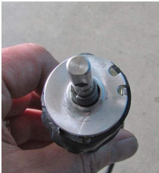
Figure 7 – Wiper Switch Clocking Spacer
