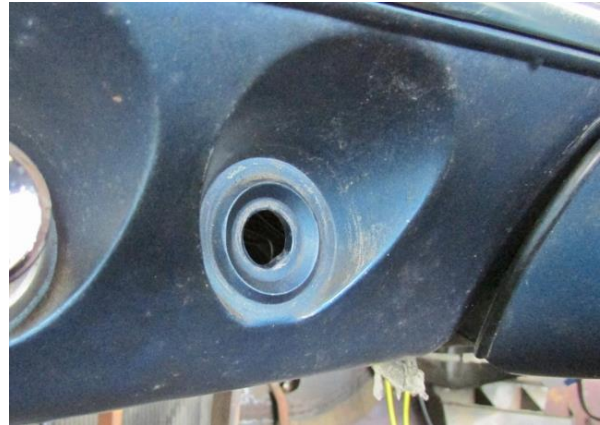
Figure 6 – Remove Factory Wiper Switch
