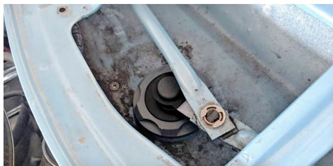
Figure 5 – Attach Wiper Linkage to Pitman Arm
