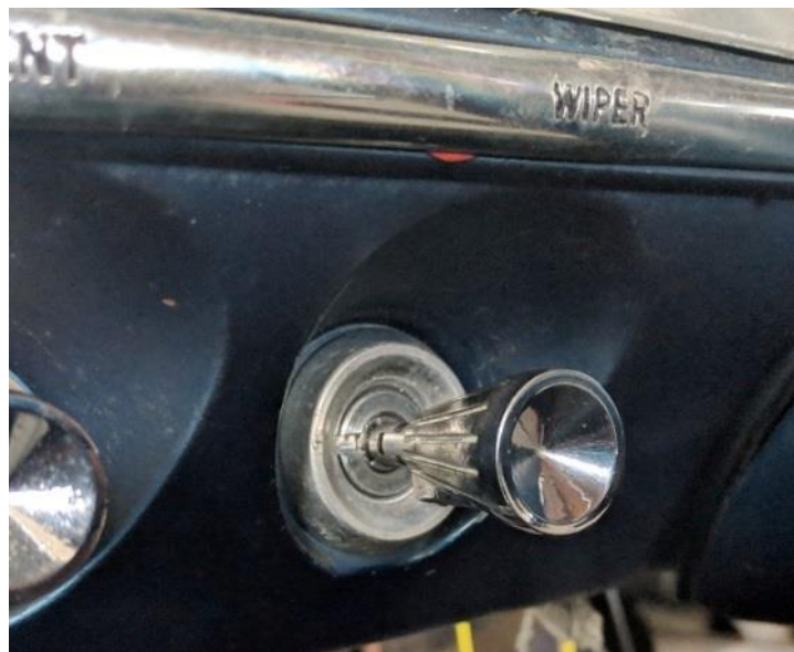
Figure 11 – Install Wiper Knob
