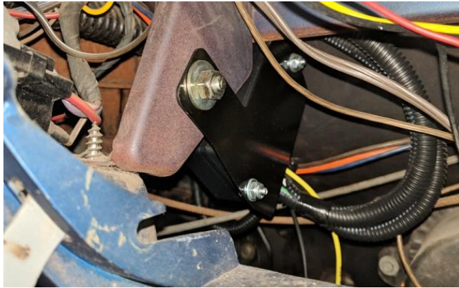
Figure 16 – Install Control Module
