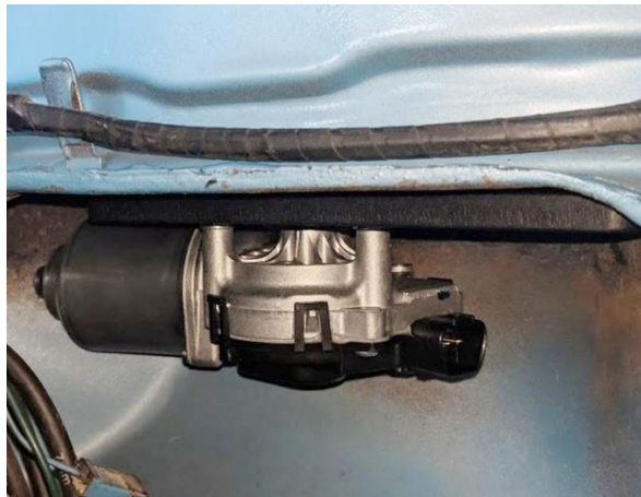
Figure 3 – Mount Wiper Motor
