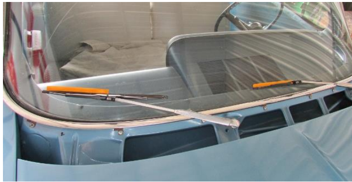
Figure 1 – Remove Wiper Arms & Cowl Panel
