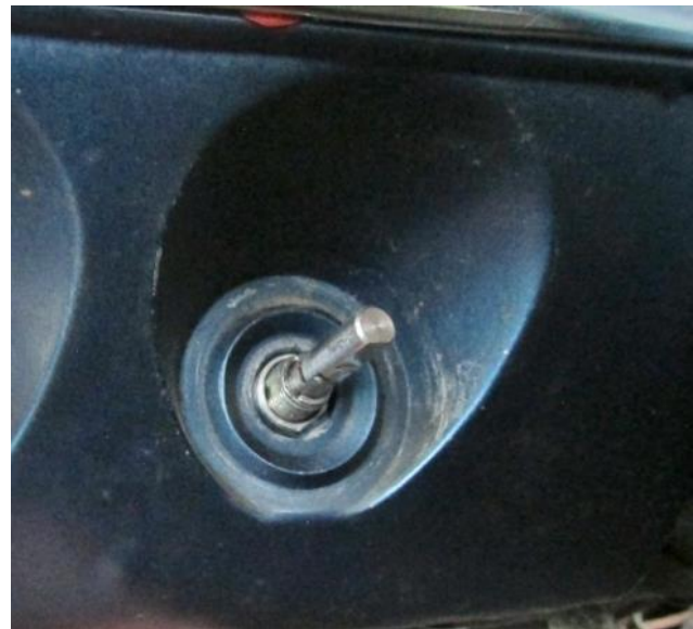
Figure 8 – Install Wiper Switch
