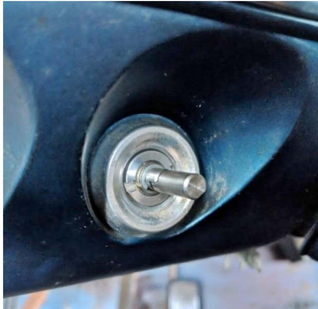
Figure 9 – Wiper Switch Retaining Nut
