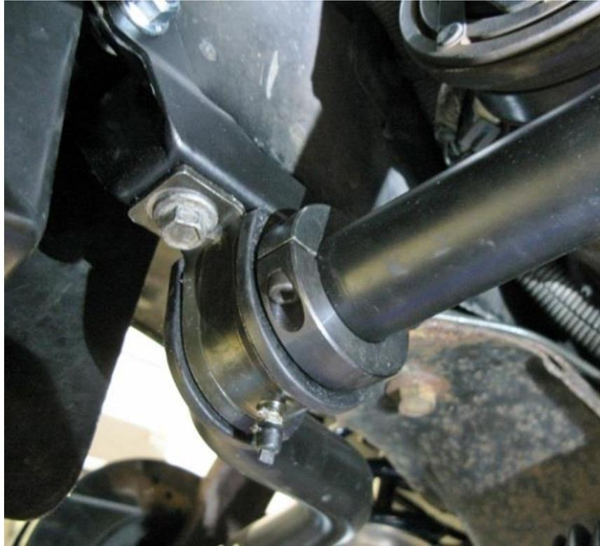
Figure 7 – Install Split Lock Collars
