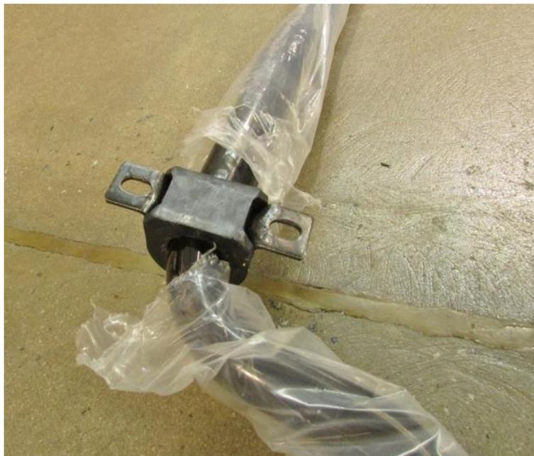
Figure 2 – Install the Urethane Bushings & Brackets
