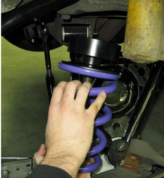
**Figure 3 - Install Weight Jack Assembly**
