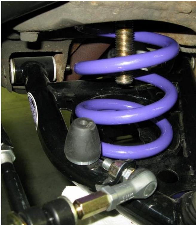
**Figure 4 - Weight Jack Assembly Installed**
