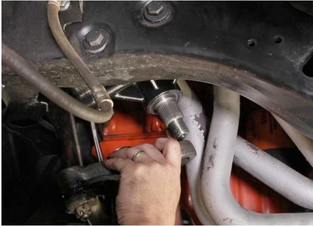
Figure 15 – Install Pitman Arm
