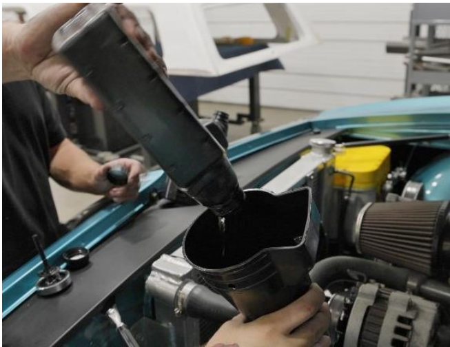
Figure 15 – Add Power Steering Fluid
