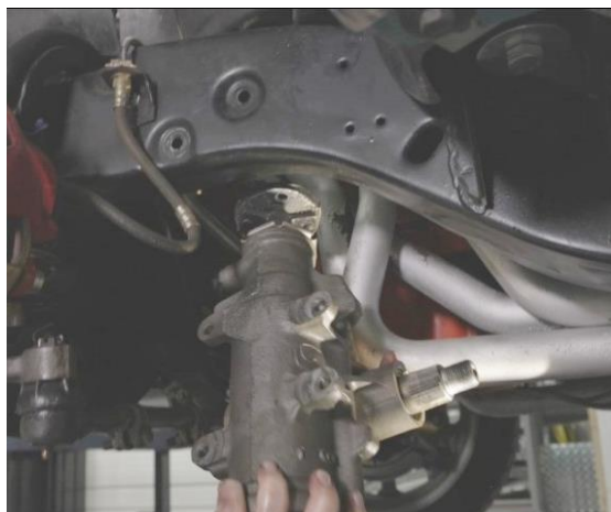
Figure 4 – Remove Steering Gear
