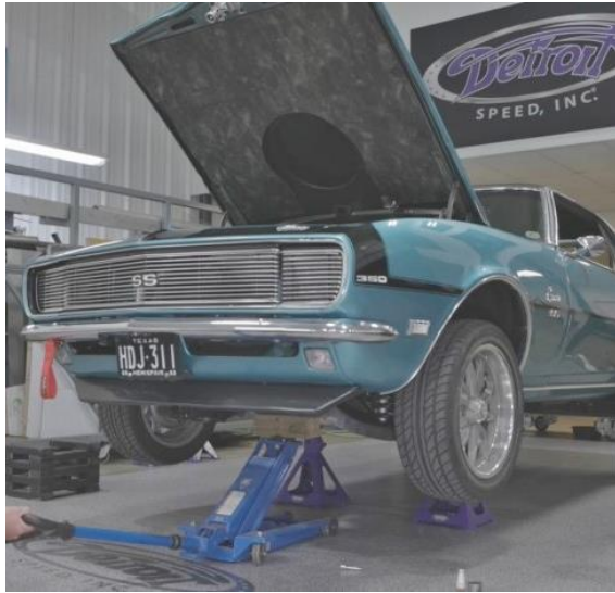
Figure 1 – Remove Driver's Side Wheel
