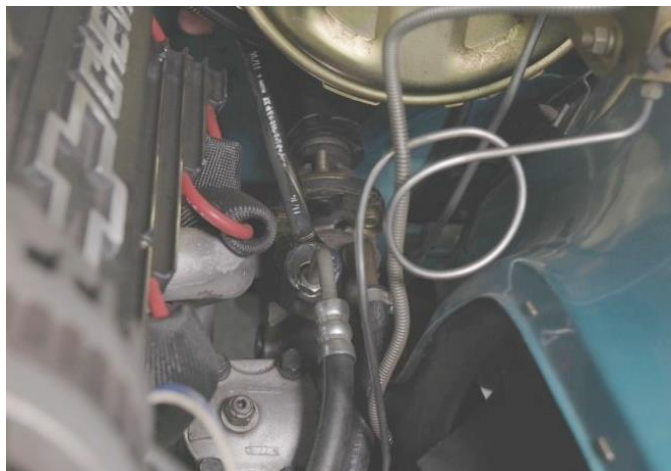
Figure 3 – Disconnect Power Steering Hoses
