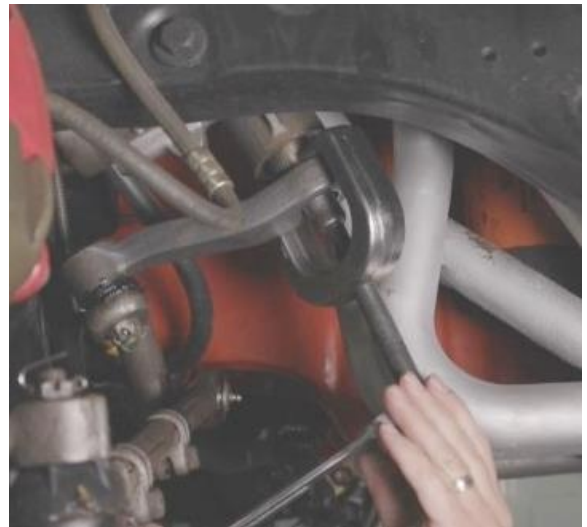
Figure 2 – Remove Pitman Arm
