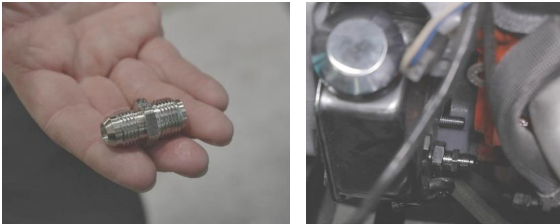
Figure 6 – Install P/S Pump Fitting
