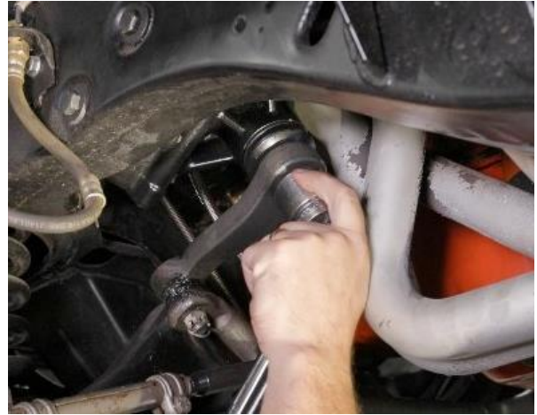
Figure 15 – Install Pitman Arm
