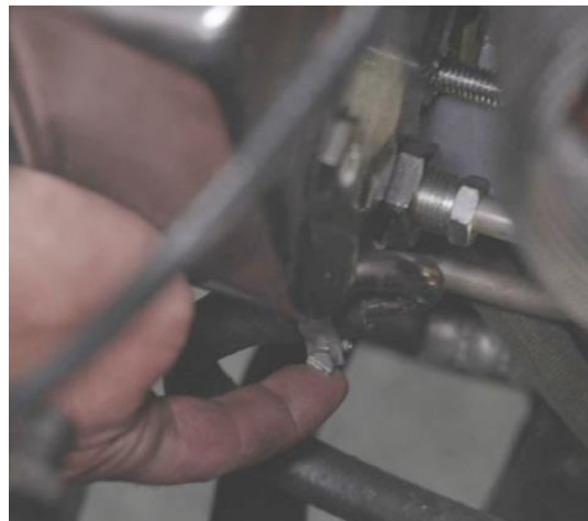
Figure 5 – Remove Pressure & Return Hoses from Pump
