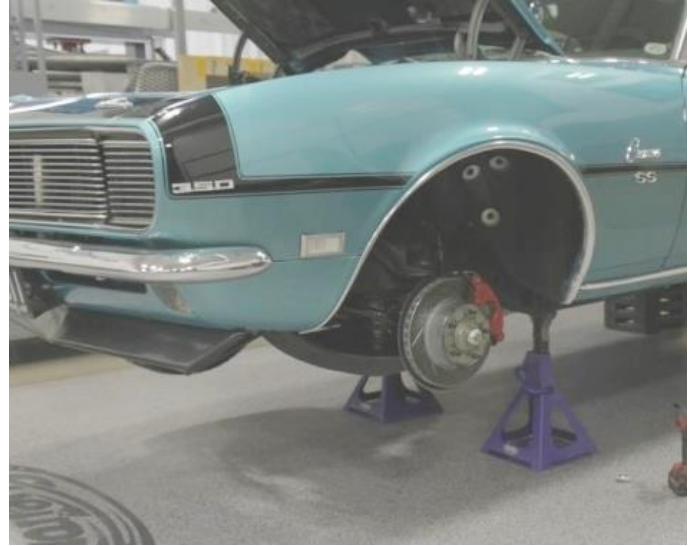
Figure 1 – Remove Driver's Side Wheel
