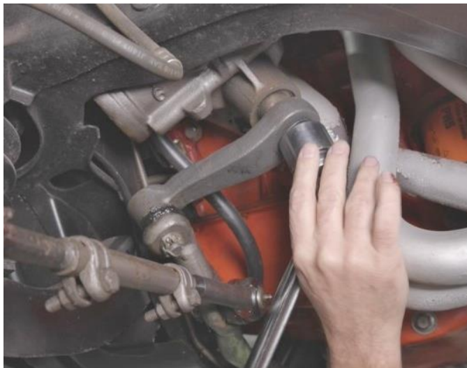
Figure 2 – Remove Pitman Arm
