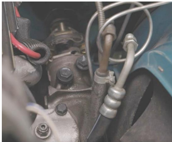
Figure 3 – Disconnect Power Steering Hoses
