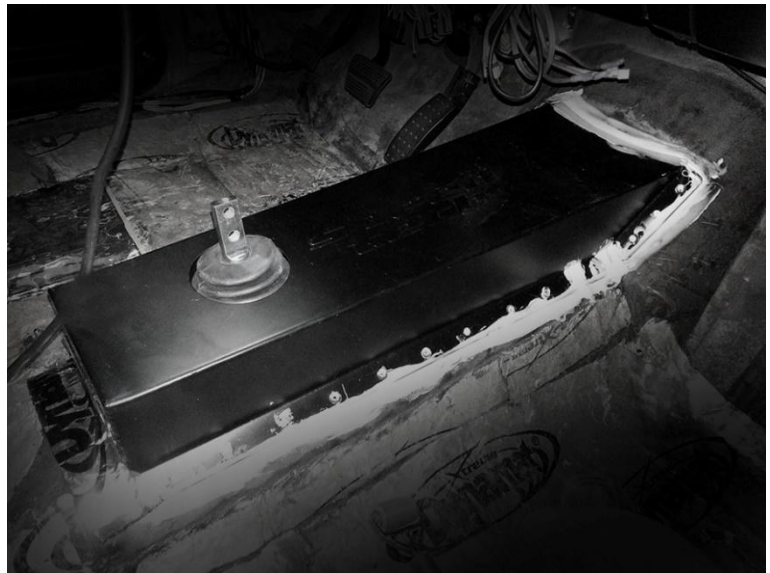
Figure 8: Seam sealing in a 1970 Nova
