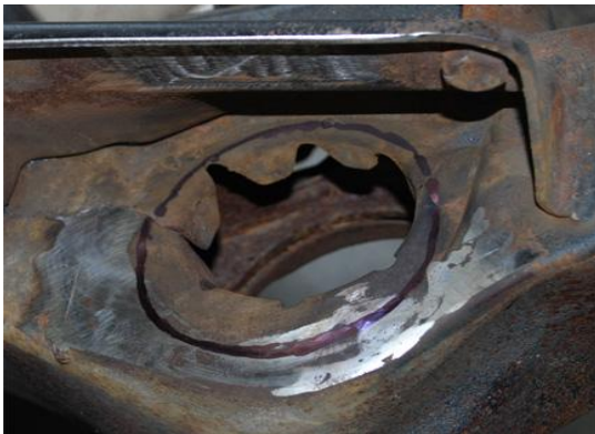
Figure 5: Cut line for the inner spring cut and the final product
