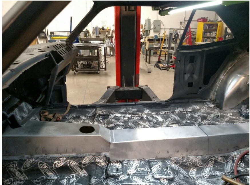
Figure 9: Result of the floor tunnel
