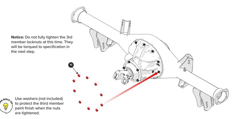
Attention: Due to the pinion yoke offset, two nuts can only be accessed with an open-end or crowfoot wrench. A crowfoot can be used with a torque wrench to set the correct torque settings.
