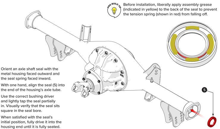
metal housing faced outward and the seal spring faced inward.
