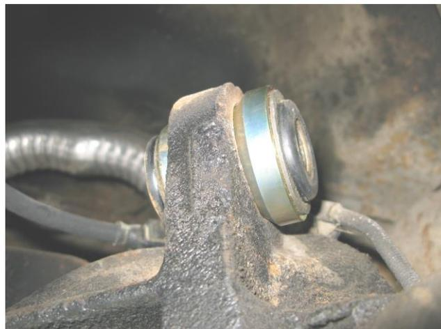
Figure 3 - Replacement Bushing Installed
