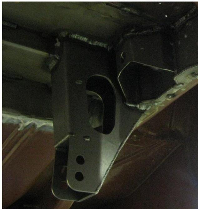
**Figure 7 - Body Side Track Bar Bracket**
