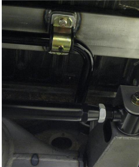
**Figure 8 – ARB Spacer and Bracket**
