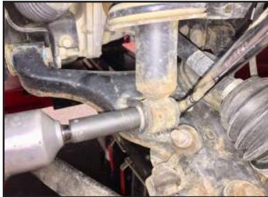
**STEP 10:** Loosen and remove three upper strut mounting nuts.
