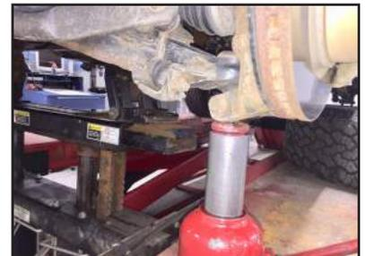
**STEP 5:** Disconnect ABS/ vacuum line brackets, if equipped, to allow slack.
