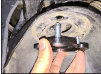
**STEP 19:** Install Jam Nut Spacer followed by Jam Nut and Snap Ring. After final height adjustment tighten Jam Nut and reinstall bracket removed in Step 15. **\*\*TIP\*\* To aid in future adjustments; coat threads between Jam Nut and Inner Adjustment Screw with anitseize.**
