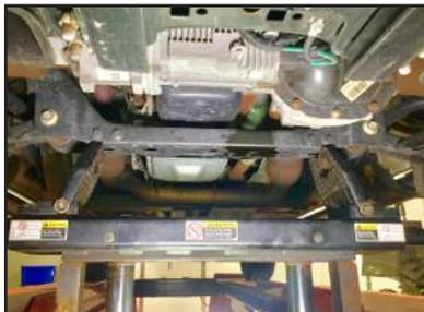
**STEP 4:** Remove front wheel and support lower control arm with floor or bottle jack.
