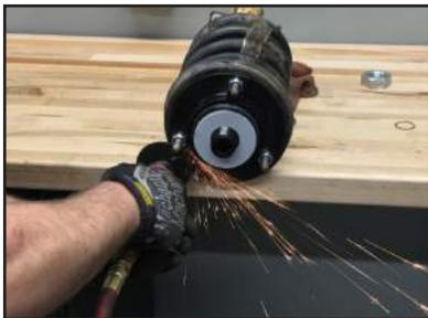
**STEP 14: \*IMPORTANT\*** Before reinstalling strut assembly make sure to install white tear-resistant nylon bearing plate!
