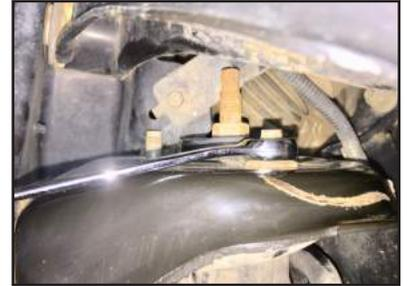
**STEP 11:** Carefully swing knuckle assembly out of the way, taking care to not over extend axle. Slowly lower jack set in Step 4. Remove strut assembly.
