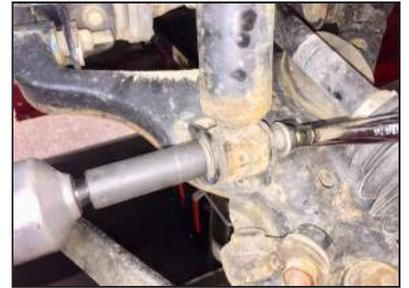
**STEP 22:** Reinstall ball joint nut and torque to manufacturer's specifications. Install new cotter pin (not included).
