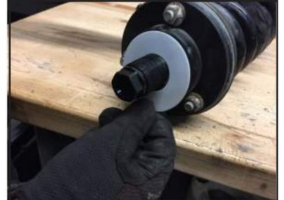
**STEP 15: IMPORTANT!** Be sure the Threaded Adjustment Screw Rotates FREELY after securing kit to the OEM strut. If not, slightly loosen the three upper stud nuts and rotate the Threaded Adjustment Screw slightly UPWARD. Re-torque upper stud nuts to OEM specifications and recheck that the Threaded Adjustment Screw now rotates properly for adjustment after installation. **If this is skipped the kit will not adjust after installation!!**
