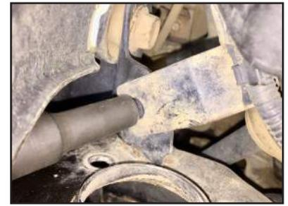
**STEP 18:** Rotate strut assembly 180\* and install into vehicle.
