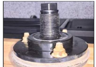
**STEP 13:** Trim strut mounting studs flush with top of OEM nut.
