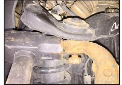
**STEP 9:** Loosen and remove lower strut bolt and nut.
