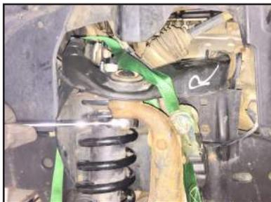
**STEP 23:** Reinstall Tie rod nut, torque to manufacturer's specifications. Install new cotter pin (not included). Reinstall sway bar end link and torque to manufacturer's specifications.
