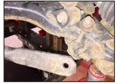
**STEP 7:** Remove tie rod end cotter pin. Loosen but don't completely remove the nut. Leave it on to protect the threads, but loose enough to remove with your fingers. Use hammer or joint removal tool to separate the taper.
