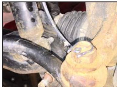
**STEP 16:** Remove bracket on top of strut tower. Retain hardware for reinstallation.
