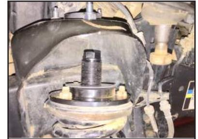
**STEP 20:** Reinstall lower strut bolt and nut. Torque to manufacturer's specifications.
