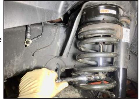
**IMPORTANT!** Check all fasteners for proper torque. Check to insure there is adequate clearance between all rotating, mobile, fixed and heated members. Check steering for interference and proper working order. Test brake system.
