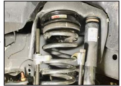
**STEP 17:** Install shock extensions using supplied hardware. Torque to 90 ft/lbs.
