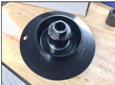
**STEP 12:** Install OEM isolator on Lift Machine. Make sure to place nub into the hole on Top Plate.
