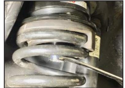
**STEP 21:** With Jam nut slightly loosened, insert 1/2" Drive extension and ratchet. Turn Inner Adjustment Screw counter-clockwise (LEFT) with ratchet to desired height. **NOTE:** Actual height of kit will be actual height of lift.
