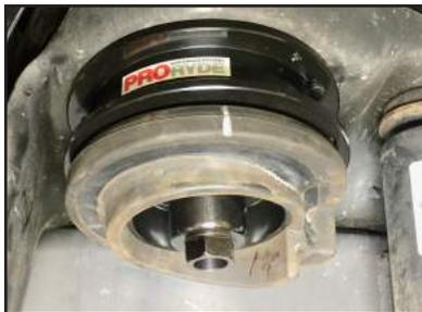
**STEP 14:** Tighten press fit studs with supplied nuts.
