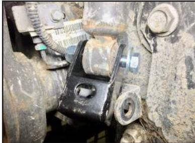
**STEP 18:** Lift axle with jack and rotate extension so nut is on frame side and tighten lower mount with OEM hardware. Torque to OEM Specifications.
