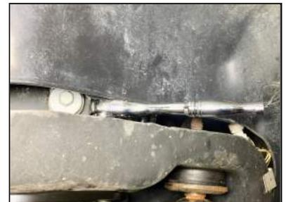
**STEP 15:** Note this picture is showing kit adjusted one thread above lowest position. Make sure kit will adjust before going further!
