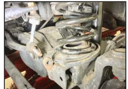
**STEP 5:** Supporting the front axle with suitable jack, disconnect lower shock bolt. Save OEM fastener for use in Step 18.
