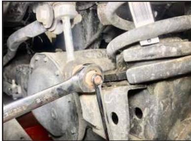
**STEP 20:** To adjust, loosen Jam Nut with 1" wrench one turn. **Do not remove!**
