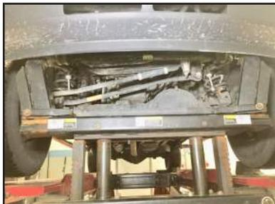
**STEP 4:** Remove sway bar end links. Disconnect ABS/Vacuum lines from bracket to allow slack.
