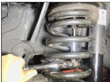
**STEP 22:** Once final height adjustment is reached, tighten Jam Nut with 1" wrench.
