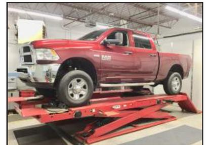
**STEP 25:** Lower the vehicle, jounce suspension and measure ride height of EACH SIDE of the vehicle, front & rear. Measure from the bottom of the wheel/rim to the lip of the fender.
