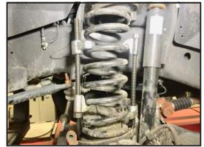
**STEP 7:** Remove Isolator and Locate OEM holes in spring mount.
