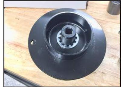
**STEP 11:** Install Jam Nut. Do not tighten yet.
