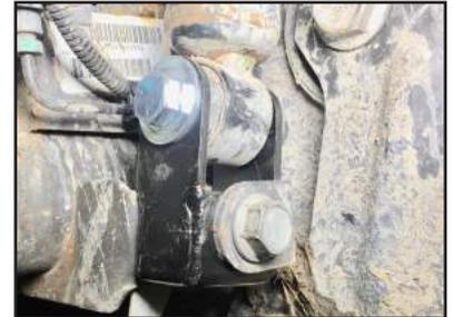
**STEP 19:** Reinstall sway link and tighten to manufacturer's specifications.
