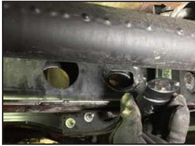
**STEP 16:** Install new Forged 3" 12.9 Adjuster Bolt make sure it has full thread engagement before releasing tension.
