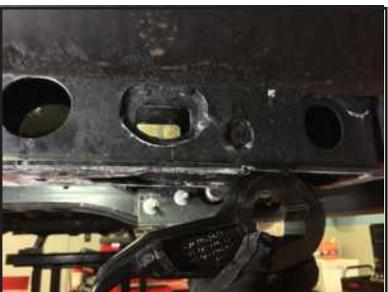
**STEP 14:** Use a Torsion Bar Loading/Unloading tool (**PRORYDE Part # 88-8000**) to compress the key until it clears the Adjuster Bracket slot.
