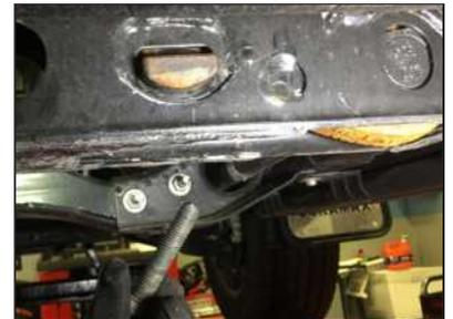
**STEP 11:** Remove both OEM Adjuster Brackets.
