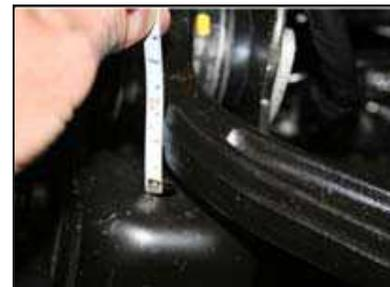
**The gap between the Upper Control Arm and Bump Stop should be 1/4" to 1/2" with weight on the wheels.**
