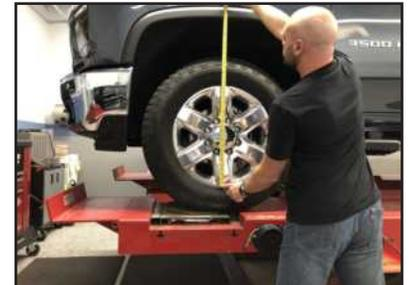
**STEP 23:** Perform a complete wheel alignment, utilizing a Certified Alignment Technician with experience working on lifted vehicles.
