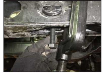
**STEP 17:** SLOWLY release tension on the Torsion Loading/Unloading Tool (**PRORYDE Part # 88-8000**) until it can be fully removed, then repeat Steps 12 through 16 on other side of vehicle.
