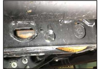
**STEP 9:** Loosen both OEM Torsion Key Adjusting Bolts.
