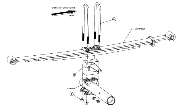
DRIVER SIDE ASSEMBLY SHOWN – 5.0" REAR BLOCK KIT: FORD F-250/F-350 SRW (with AUX SPRINGS)«
