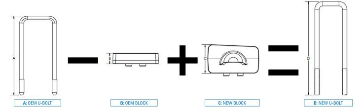
If the sum of measurement  $\bf A$  and  $\bf C$ , minus measurement  $\bf B$ , is equal or less than to the length of the new U-bolts ( $\bf A-B+C=D$ ), then you can proceed with the installation.
