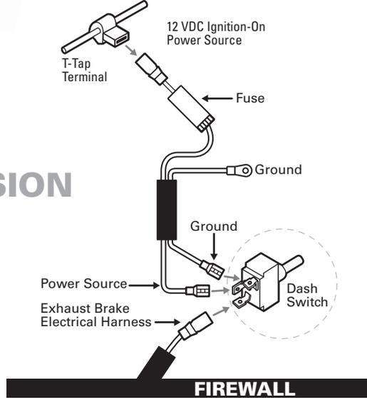
EXHAUST BRAKE CONNECTIONS WITH OPTIONAL SWITCH-PAC
