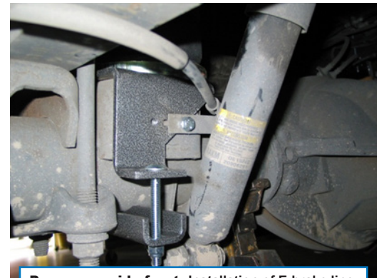
Passenger side front. Installation of E-brake line.
