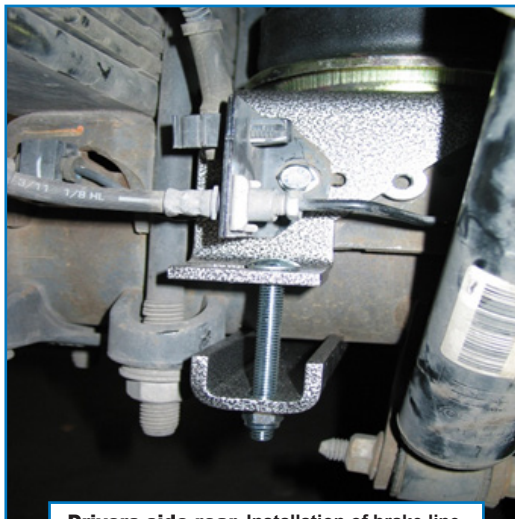
Drivers side rear. Installation of brake line.
