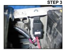
Locate the black wire of the relay harness, route it to the air tank location.
