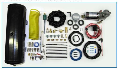
**IMPORTANT:** These kits include push-to-connect airline fittings. They require the end of the airline to be cut cleanly and square to ensure the internal seal will not leak air. The airline must only be cut with a sharp knife or hose cutter. Using scissors or wire cutters will distort the airline causing the connection to leak air past the o-ring seal.
