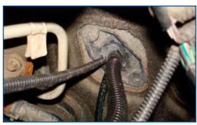
Locate the factory 3 Pin Weather-Pac connector on the the driver side of the engine (shown by the arrow). Remove the protective cap and install the mating connector in the Pacbrake harness. Install the protective cap removed on the unused connector on the Pacbrake harness. If you have a performance module connected to the 3 pin weather-pac, simply insert the Pacbrake connectors between the factory connector and the performance module connector. Secure wires with the tiestraps provided.
