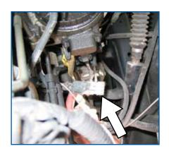
Mount the Pacbrake control unit to the aluminum bracket on the inside of the firewall as shown in the photo using the fasteners supplied.
