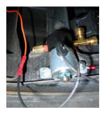
Remove the lower dash panel below the steering column. Locate the plastic plate in the driver side of the firewall. Drill a hole large enough to feed the Pacbrake harness through, then feed the harness into the engine compartment from the cab side. Once the harness is positioned and secured apply silicone around the loom to provide a seal. Connect the orange wire to the remaining solenoid wire, crimp the connector to the wire, then heat the connector to provide a water-tight seal.
