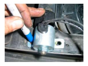
Using the fittings and nylon airline provided, source supply air from the tank, connect to solenoid port marked "IN". Connect the solenoid port marked "CYL" to the air cylinder on the exhaust brake. Secure the airline with the tie-straps provided.
