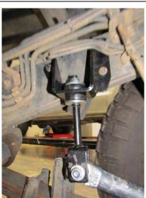
3. CONNECT THE SWAY BAR LINKS TO THE DROPPER BRACKETS ALLOWING THE SWAY BAR TO HANG UNDER THE VEHICLE. TIGHTEN UNTIL NUT BOTTOMS OUT.
