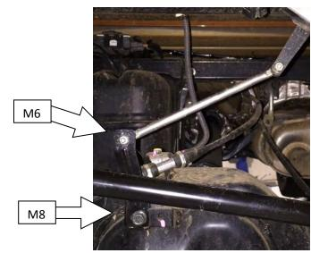
Install new pot extension bracket 3759727 re-using OE fasteners back to their original location and also new M8 bolt and flat washer in the right lower hole of the new bracket.
