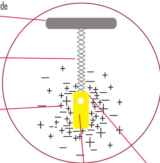
Magnesium anode with protective shield.
