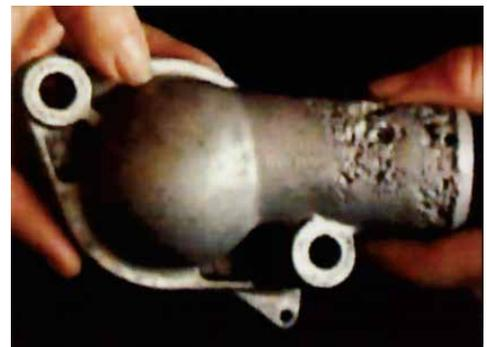
Without Sacrificial Anode Radiator Cap, the thermostat housing cover shows major deterioration after 60,000 miles.
