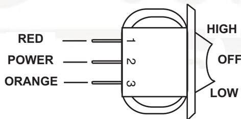
NOTE: The low speed terminal is located behind the high position due to internal switching.
