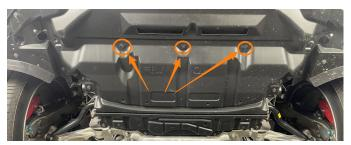
**3.** Remove 16x 10mm bolts and remove the undertray from the vehicle.
