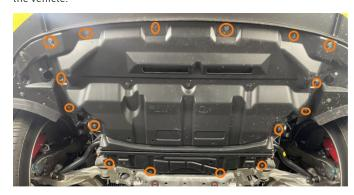
4. Thread 4x included M6 bolts and washers in the rear-most bolt holes 1-2 turns.
