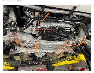
5. Install skid plate. First, align the rear skid plate slots with the four bolts installed in step 4 and raise the skid plate. Install 1-2 of the factory front bolts to hold the skid plate in place. Then, thread the rest of the OEM bolts through the skid plate. Leave all bolts loose until all 16 bolts are started. Make sure that the wire harness shown in the picture in step 4 is not pinched between the aluminum bar and the skid plate. [Image on next page]
