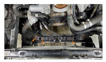
6. Be sure to reinstall the lower radiator mount grommets into the vehicle if they stayed attached to the stock radiator during removal. Install the Mishimoto radiator into the lower radiator mounts. Then, using pliers or a remote-action hose clamp tool, install the lower radiator hose onto the Mishimoto radiator. For vehicles with an automatic transmission: Install the transmission lines into the fittings for the internal transmission cooler on the Mishimoto radiator. (Image on next page)
