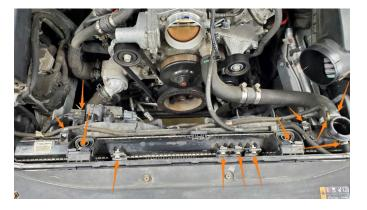
5. Using pliers or a remote-action hose clamp tool, remove the lower radiator hose. For vehicles with an automatic transmission: Remove the dust covers from the internal transmission cooler lines. Then, using a pick or a 3/8" transmission line disconnect tool, remove the internal transmission lines from the radiator. Be prepared to catch any transmission fluid that may leak out in an appropriate container and dispose of it properly.
