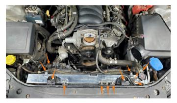
**8.** Reinstall the intake and tighten the throttle body and air box hose clamps. Then, reconnect the MAF sensor plug and breather hose that were disconnected in step 3. [Image on top right]
