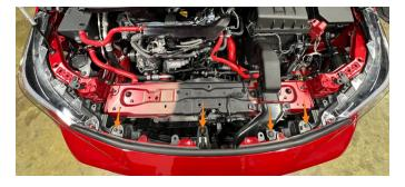
7. Disconnect the electrical connector from the ADAS radar in the center of the bumper. Then, carefully pull each end of the bumper away from the vehicle to begin to disconnect it. Disconnect the electrical connectors from the fog light on each side of the bumper before entirely removing the bumper.
