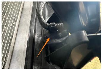
**14.** Remove the left and right plastic shrouds by pulling straight out until the clips disengage and the shrouds are free.
