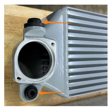
**19.** Using a silicone-based lubricant, lubricate the 0-rings on the intercooler inlet and outlet adapters.
