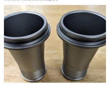
20. Carefully press the inlet and outlet adapters into the intercooler 0-ring grooves. Place the locking rings over the flanges. Using a 8mm socket, secure the locking rings with the four (4) included bolts. Torque the bolts to the specified torque, do not over tighten.
