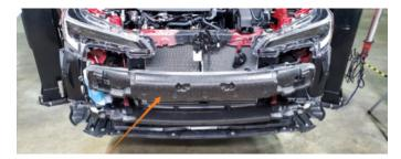
10. Using a 10mm socket, remove the nut that attaches the bracket to the bottom center of the crash bar. Then, unclip the plastic wire harness mount from the top of the crash bar. Then, using a 14mm socket, remove the eight (8) bolts that secure the crash bar and remove the bar from the vehicle. During reassembly torque the crash bar bolts to 49 ft-lb (67Nm).
