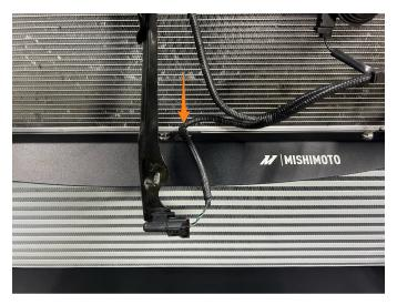
**24.** Install the Mishimoto lower intercooler shroud. Using a 10mm socket, secure the shroud with the three (3) included bolts.
