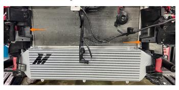
23. Install the Mishimoto upper intercooler shroud. Use a 10mm socket to install the three (3) included bolts. Reinstall the two (2) pop clips for the left and right ducts. Insert the ambient air temperature sensor tree clip into the provided hole.
