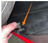
**5.** Remove the seven (7) pop clips securing the plastic tray at the front of the engine bay and remove the tray from the vehicle.
