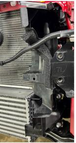
**15.** Loosen the hot side and cold side intercooler coupler clamps. Disconnect the couplers from the intercooler.
