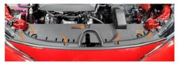
**6.** Using a 10mm socket, remove the three (3) bolts securing the top of the bumper to the vehicle. Then, remove the pop clip securing the snorkel duct.
