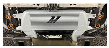
**33.** Secure the intercooler to the brackets using the provided 12mm bolts. (2x HF8X1.25-25A)
