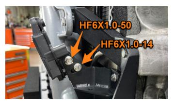
**49.** Using a square with a bubble level, adjust the sensor pivot angle until it is level. Once the sensor is level, tighten the bolts.
