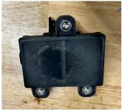
**47.** Install the MM2420-02 bracket to the driver-side intercooler mounting bracket using the provided hardware. (2x HF6X1.0-14)
