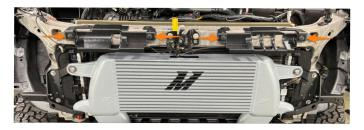
38. If your vehicle is equipped with the modular bumper, fasten MM1867-02 to the upper intercooler bracket, ducting, and foam assembly using the provided pop clips. (4x MM930). \*Proceed to step 39 if your vehicle is not equipped with the modular bumper.
