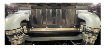
**68.** Remove the stock intercooler quick disconnect adapters and boots. (4x MM1533-92 clamps)
