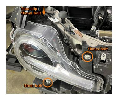
13. Using a screwdriver or pick tool, release the barb securing the headlight to the radiator active grille shutter assembly. Once removed, disconnect the electrical harness connector.
