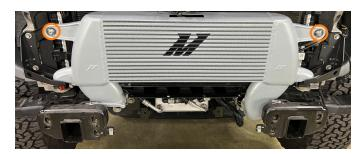
**34.** Pull outward on the upper intercooler mounting bracket, ducting, and foam assembly until the  $\frac{1}{2}$  mounting holes align with the threaded holes in the frame. Once aligned, use the original fasteners to secure it in place. (2x 15mm bolts) (Images on next page)
