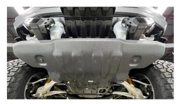
**79.** Guide the front bumper back onto the vehicle, ensuring that the lower intercooler ducting slides into the upper area of the bumper.
