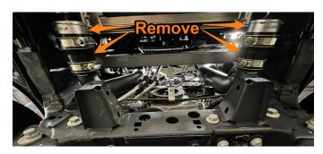
**69.** Using the MM4634-01 extended boots, connect the Mishimoto intercooler piping to the inlet and outlet of the intercooler.
