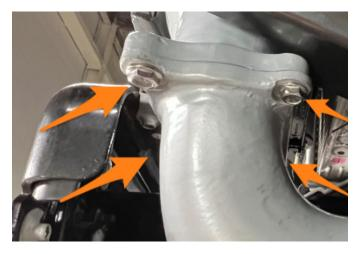
**66.** Assemble the provided adapters and couplers with the provided clamps. (2x MM1853-01, 2x MM4618-01, and 2x MM1533-92)
