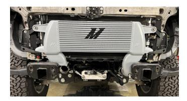
**32.** Install the remaining bolts to secure the intercooler brackets to the vehicle, then tighten them. (2x 10mm bolts)
