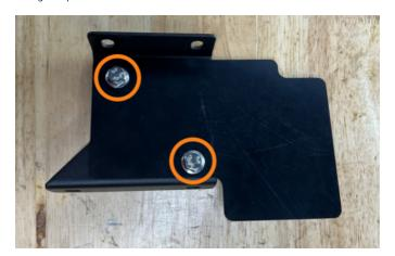
**62.** Install the MM2392-04 bracket to the passenger-side intercooler bracket using the provided hardware. (2x HF6X1.0-12A) (Image on top right)
