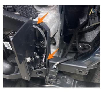
**56.** Unseat the connector from the driver-side of the radiator grille shutter assemble.
