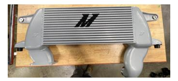
**31.** Maneuver the driver-side of the intercooler between the frame and ducting, then lower the passenger-side of the intercooler down between the frame and A/C condenser. Once the intercooler is in its approximate location, rotate the brackets into position and lower the intercooler into the brackets. (Image on top right)
