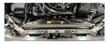
04. Locate the front two rotating fasteners securing the fender flares in place and turn them 90 degrees, then pull outward to partially remove them. Do this on both sides.
