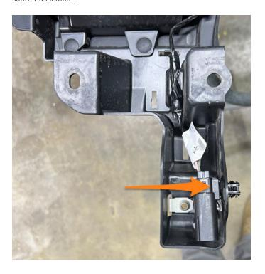
**57.** Remove the connector tree clip from the connector using a panel tool or flat head screwdriver.
