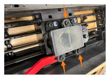
**45.** Remove the 3x plastic bushings from the sensor by pushing the tabs inward while applying some downward pressure, then push the bushings out of the sensor brackets.
