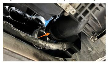
8. The aluminum reinforcing plate can be removed to make the next step much easier on the M2 model. Position the coupler on the pipes from the bottom so it is centered between the beads. Arrange the clamps on the coupler so they are centered between the bead "bump" and the end of the coupler. Then, use an 8mm socket and long extension to tighten the 2 clamps from below.
