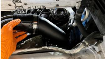
**5.** Ensure the peg is aligned with the bushing (A) then push the quick connect (B) onto the throttle body until the spring clip snaps into the groove. Reinstall the pressure sensor into pipe 2 using the supplied M6 screws and washers. Push hose (C) onto the pipe until it clicks.
