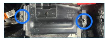
2. Slide the Bronco Direct-Fit Relay Bracket under the battery tiedown strap, as shown in the image below, then tighten the two 13mm nuts to secure it in place.
