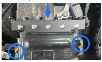
3. Using the provided M6x1.0 bolts, secure your relays to the bracket.
