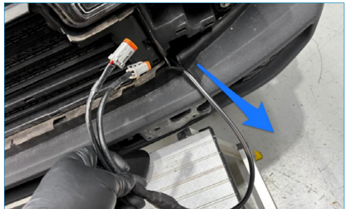
16. Once the connectors on the ends of the wire harnesses make it past the bottom of the grill support structure, carefully pull on the wire harnesses until the slack in the engine bay is removed. Proceed to step 27.
