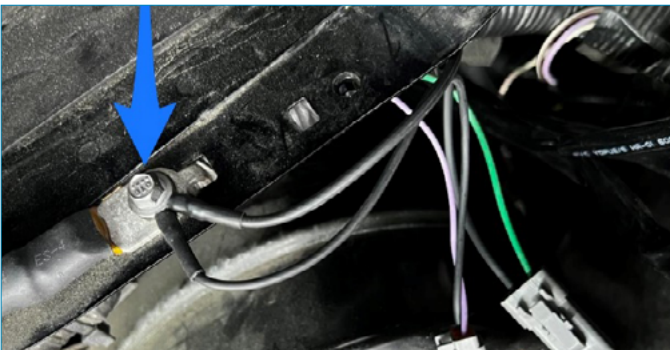
14. Connect the direct-fit wire harnesses to the connectors.
