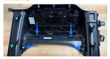
12. Remove the three 6mm screws from the backside of the climate control assembly.
