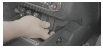
**24.** Depress the brake pedal and shift the gear selector back into park.
