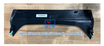
**15.** Using a file or similar abrasive tool, remove the material located in the box that was marked in the previous step. A pair of side cutters may be used as a means to quickly "rough-in" the area where the material is being removed; however, a file and sandpaper should be used to clean up all edges to create a clean-looking cut.
