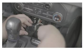
**23.** Install the provided panel plugs into the remaining empty slots on the switch panel.
