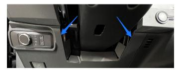
7. Remove the 7mm bolt located in the upper right corner.
