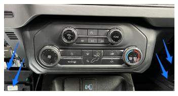
ID. Disconnect the three wire harness connectors from the backside of the climate control assembly. Once the connectors have been removed, remove the climate control assembly from the vehicle.
