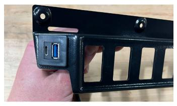
**2.** Feed the provided zip-ties through the plastic tabs on the backside of the panel-mounted USB adapter, then zip them in place. Trim the excess sections of the zip-ties for a clean finish.
