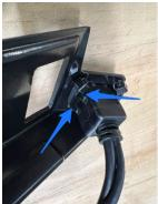
Connect the USB-A and USB-C 90° adapters to the ends of the panel-mounted USB adapter cables.
