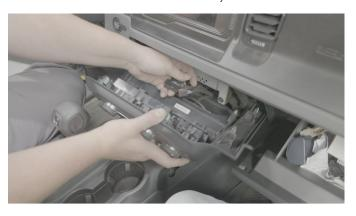
**21.** Line up the Borne Off-Road lighting/accessory wire harnesses with the notch cut out in the climate control assembly's lower trim panel, then firmly press the climate control assembly back into place.
