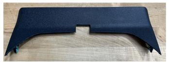
16. Reinstall the lower trim panel onto the climate control assembly.
