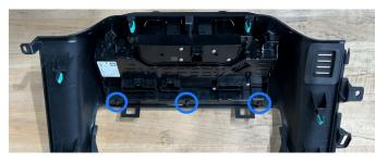
**13.** Install the Borne Off-Road switch panel and secure it in place with the three 6mm screws removed in the previous step.
