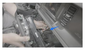
**20.** Reconnect the three previously removed harness connectors to the backside of the climate control assembly.
