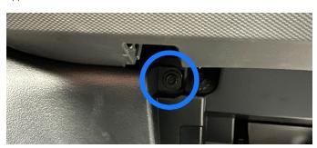
**6.** Pull outward on the driver-side dash panel under the steering column. Once all of the clips securing it in place are free, the panel will swing downwards to the floor.
